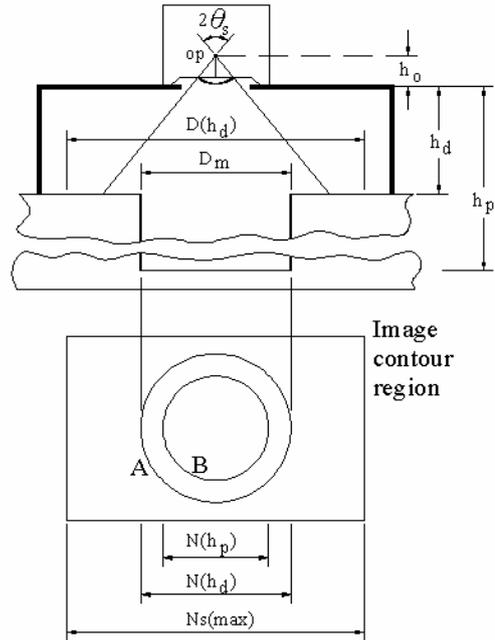
Fig. 4 Schematic diagram of measurement frame.
