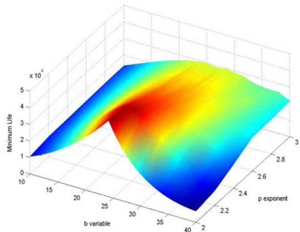
Figure 4 - Three-dimensional solution space representation for medium categorised crack length
