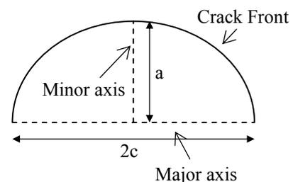
Figure 1. Semi-elliptical crack specifications
