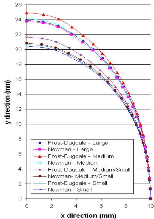
Figure 3. 2-D representation of optimised hole geometries for all cases implementing the biological algorithm.
