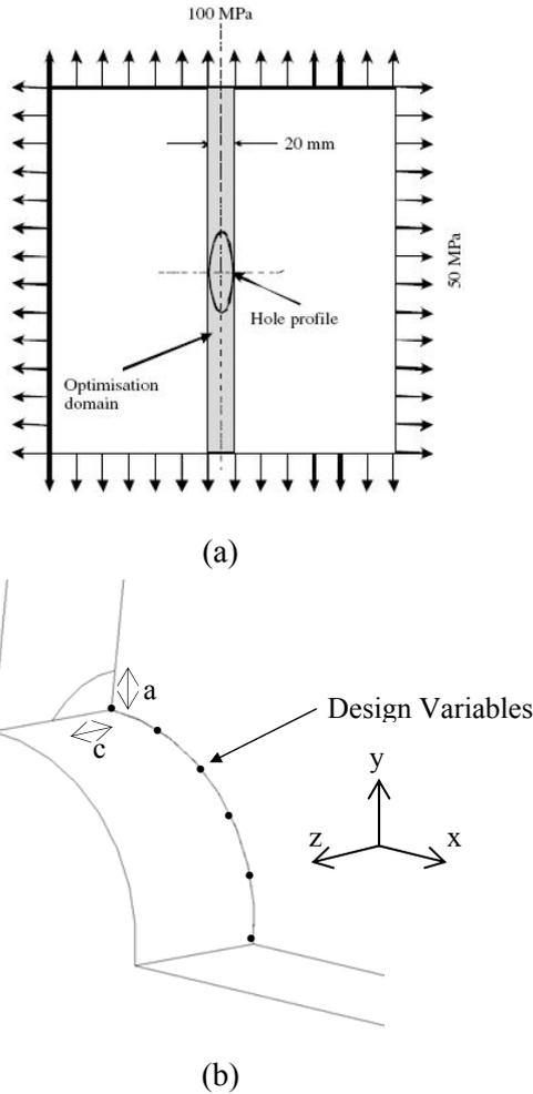
Figure 2. a) Full Schematic of the 7050-T7451 aluminium alloy. b) 1/8 model with crack specs
