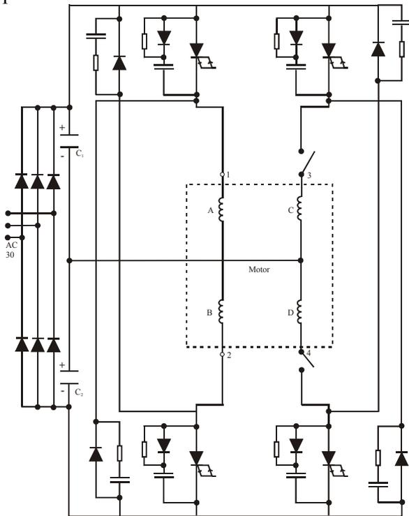
Fig. 2. Converter circuit for 4-phase SR motor, showing switches for disconnecting phases C and D (3&4).
