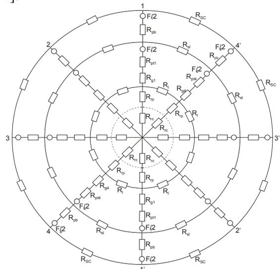
Fig. 3. Magnetic circuit model for 4-phase SR motor.
