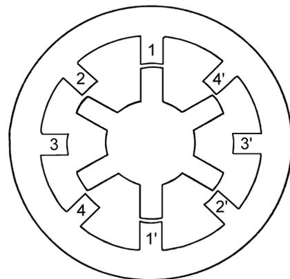
Fig.1. Schematic diagram of a 4-phase SR motor with 8/6-pole configuration.
