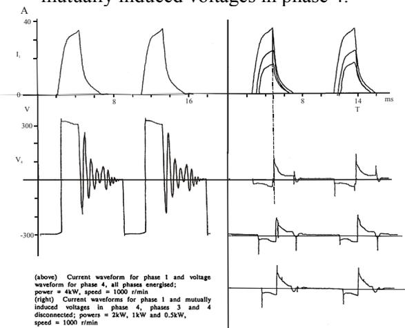
Fig. 8 Experimental waveforms at 1000 rpm with mutually induced voltages in phase 4.
