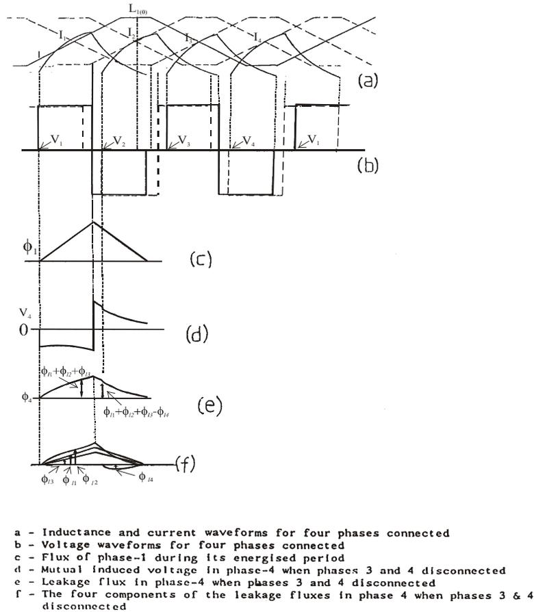
Fig. 6. Schematics waveforms based on experimental observation.
