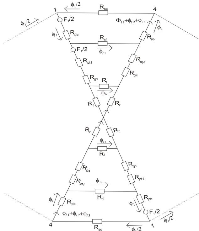
Fig. 4. Magnetic equivalent circuit with phase 1 excited and phase 4 off.
