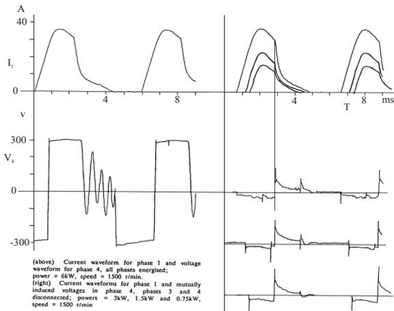
Fig. 7 Experimental waveforms at 1500 rpm with mutually induced voltages in phase 4.
