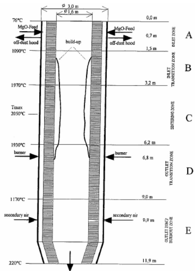
Fig.4: Schematic diagram of design temperature of the original kiln as a function of height.
