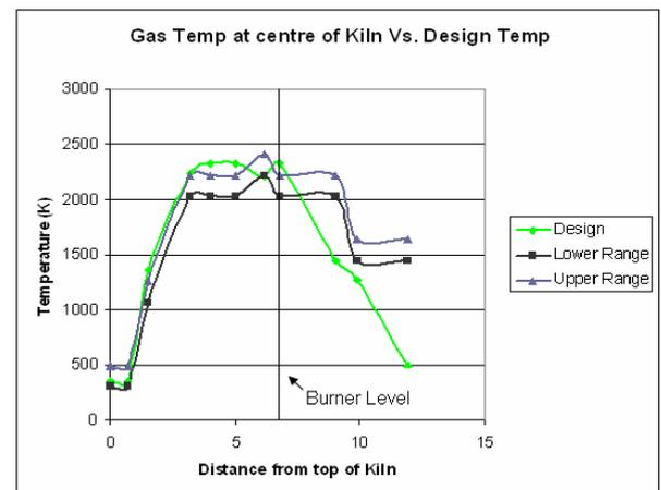
Fig.6c: Gas heat profile (Centre) vs design profiles
