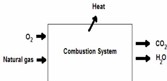
Fig.2: Schematic diagram of the simplified combustion system in the kiln
