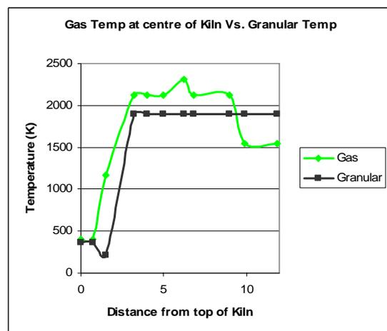
Fig.7c: Centre of kiln gas temperature vs granular temperature
