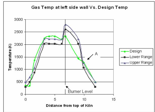
Fig.6a: Gas heat profile (left wall) vs design profiles
