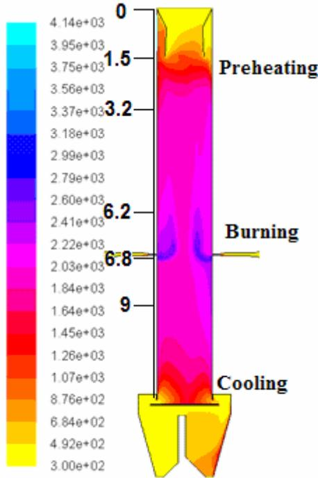
Fig.5: Contour of gas temperature at steady state
