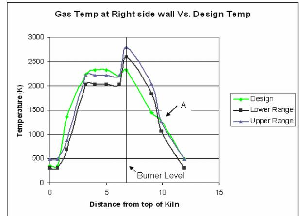
Fig.6b: Gas heat profile (right wall) vs design profiles
