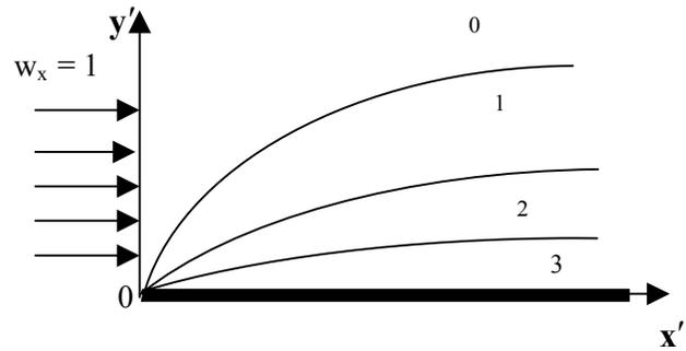
**Fig.6** Turbulent flow over a flat plate, (0) turbulent free stream (1) turbulent boundary layer at LED scale (2) laminar boundary layer at LCD scale (3) laminar sub-layer at LMD scale.
