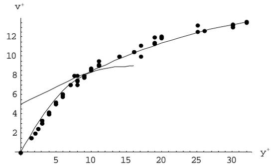
**Fig.9 Comparison between the predicted velocity profile from (62) and (63) and experimental data in the literature [37, 50, 51].**
