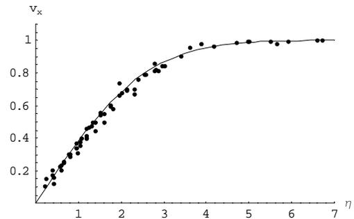
**Fig.4 Comparison between the predicted axial velocity profile from (38) and the experimental data of *Dahwan* [35].**
