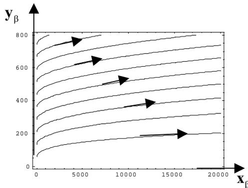
**Fig.5** Calculated streamlines from (41) for both laminar and turbulent flow over a flat plate.
