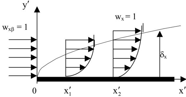
**Fig.3 Laminar boundary layer over a flat plate.**
