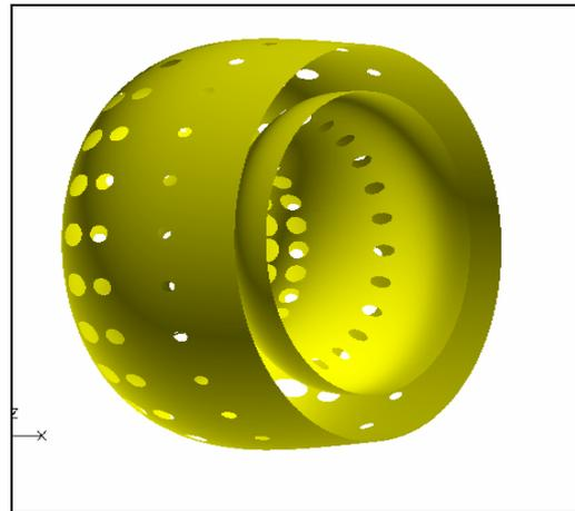
Fig. 4. Model of Flame Tube
