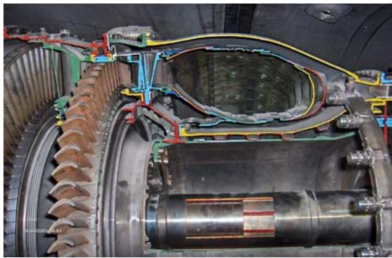
Fig. 2. Combustion chamber
