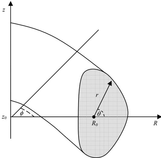
Fig. 4. Cylindrical coordinates  $(R, \phi, z)$  for the plasma and polar coordinates  $(r, \theta)$  of the poloidal section referred to the magnetic axis  $(R_0, z_0)$
