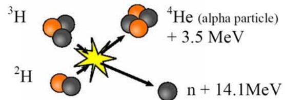
Fig. 1. Nuclear fusion reaction of Deuterium and Tritium
