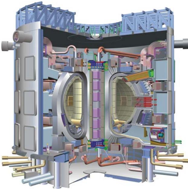
Fig. 2. ITER tokamak planned reactor (poloidal cut)
