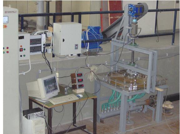
Fig. 2. Complete assembly of the experimental apparatus and the model pump.
