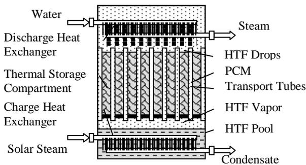
Fig. 1. Layout of the RHTS concept
