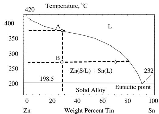
Fig. 2. Zn-Sn phase diagram
