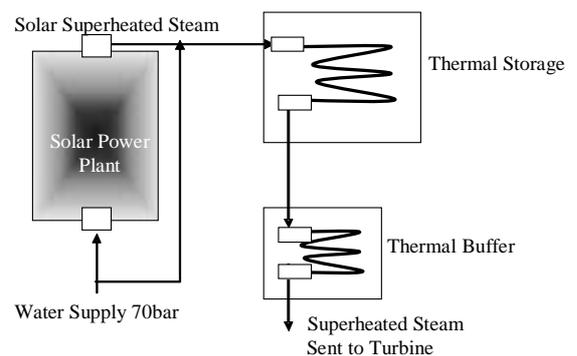
Fig. 3. Two-stage RHTS module integrated in a solar power plant.
