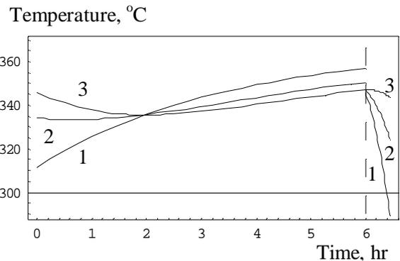
Fig. 4. Temperature variations during one continuous cycle of 6hrs charge and 1hr discharge: 1- Steam exiting main storage, 2- Steam exiting buffer, 3- Buffer PCM.
