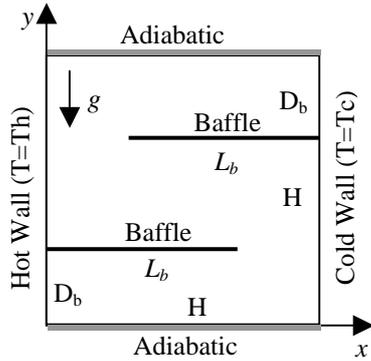
Fig.1 Schematic of the square cavity with thin insulated baffles attached to the vertical walls
