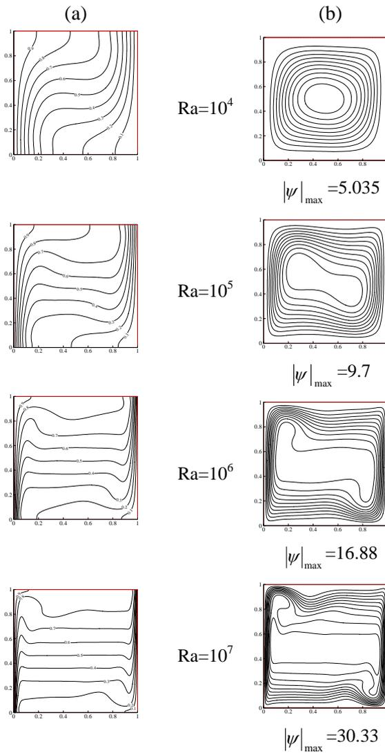
Fig.2 Isotherms (a) and Streamlines (b) of natural convection in a square cavity
