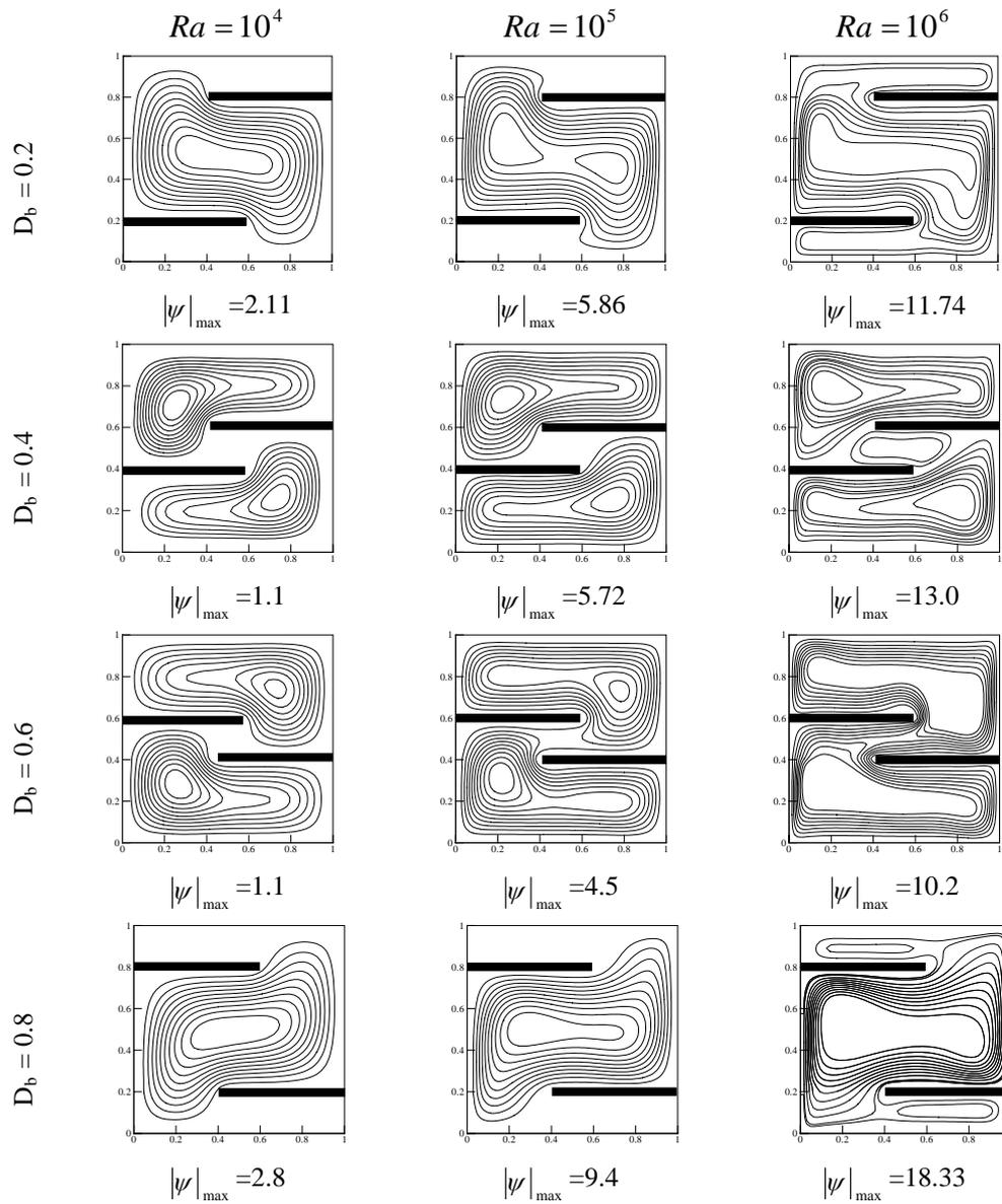
Fig.3 Streamlines for  $L_b = 0.6$  and various  $Ra$  and  $D_b$
