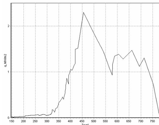
Fig. 4 Heat flux density versus surface temperature for MZM-16 oil at 61°C.
