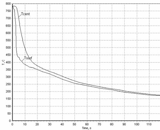
Fig. 5 Temperature at the surface and in the core versus time for MZM-16 oil at 100°C, specimen: cylinder of 9.95 mm radius and 80 mm height.
