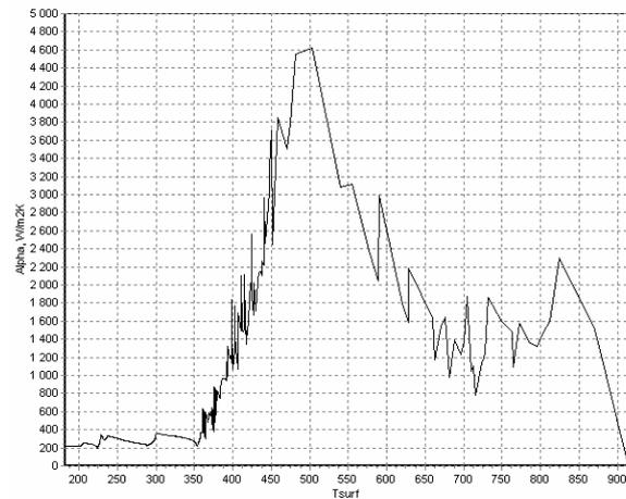
Fig. 9 Heat transfer coefficient versus surface temperature for MZM-16 oil at 170°C
