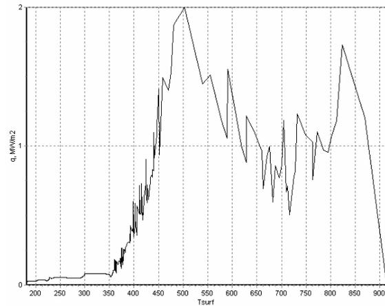
Fig. 8 Heat flux density versus surface temperature for MZM-16 oil at 170°C..
