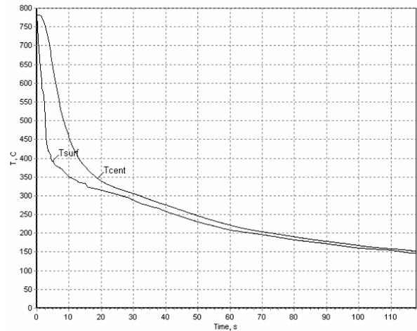
Fig. 2. Temperature at the surface and in the core versus time for MZM-16 oil at 61°C, specimen: cylinder of 9.95 mm radius and 80 mm height.
