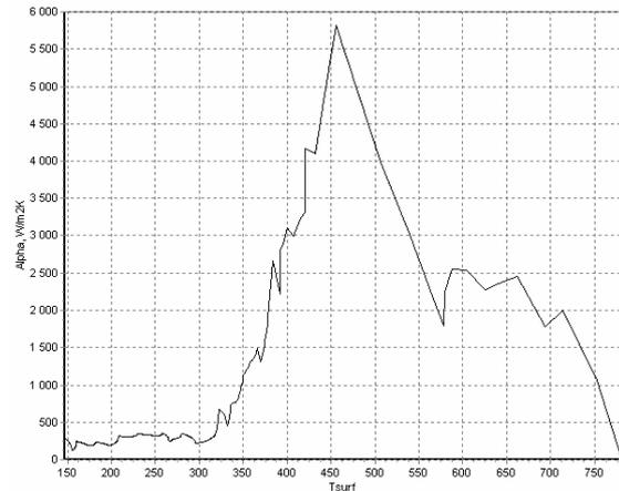
Fig. 3 Heat transfer coefficient versus surface temperature for MZM-16 oil at 61°C, specimen: cylinder of 9.95 mm radius and 80 mm height.
