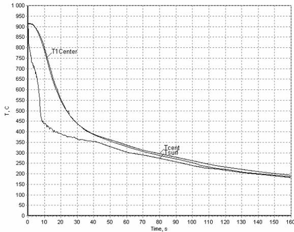
Fig. 10 Temperature at the surface and in the core versus time for MZM-16 oil at 170°C.
