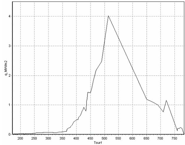
Fig. 7 Heat flux density versus surface temperature for MZM-16 oil at 100°C..
