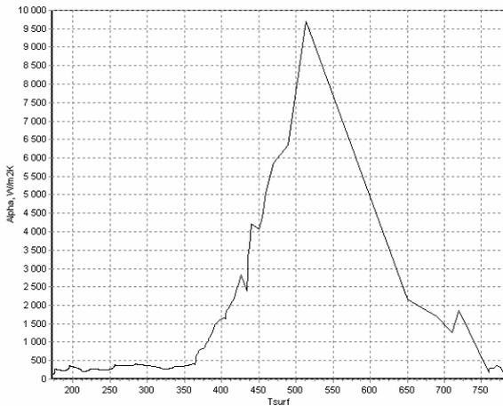
Fig. 6 Heat transfer coefficient versus surface temperature for MZM-16 oil at 100°C,
