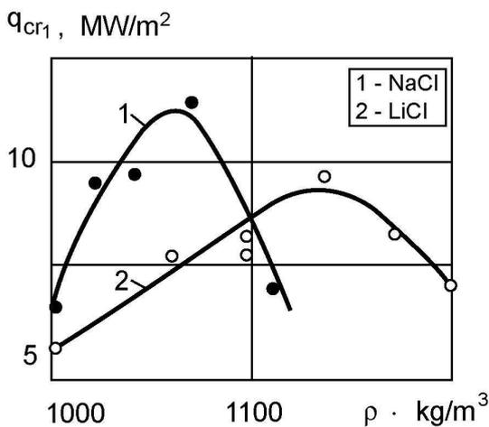
Fig. 2 First critical heat flux density  $q_{cr1}$  versus the concentration of NaCl and LiCl in water [1]
