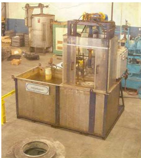
Fig. 4 Single-part quenching IQ system
