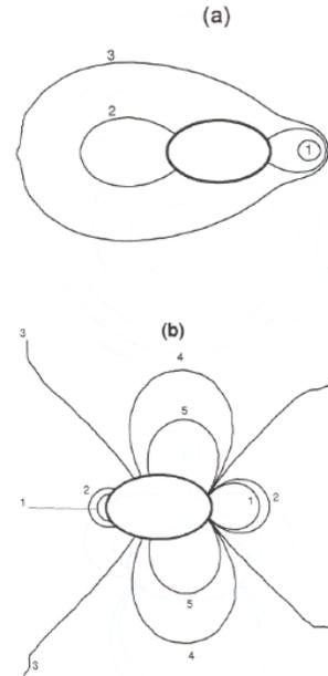
Fig. 3: The numerically obtained streamlines and vorticity pattern for  $c = 2.236$  with  $N = 800$ . (a) the streamlines labeled 1, 2 and 3 correspond to  $\psi = -0.65, 0.00$  and  $0.19$ , respectively, (b) the vorticity lines labeled 1, 2, 3, 4 and 5 correspond to  $\omega = -0.07, 0.0, 0.22, 0.3$  and  $0.4$ , respectively.
