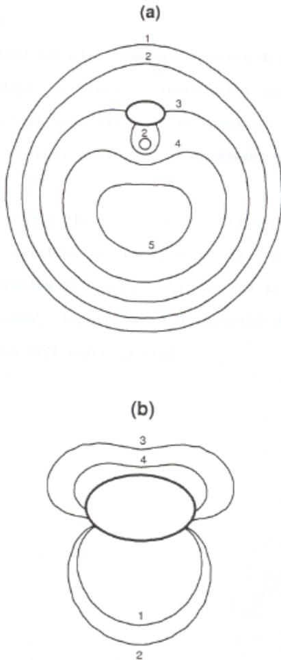
Fig. 4: The numerically obtained streamlines and vorticity pattern for  $c = 2.236$  with  $N = 800$ . (a) the streamlines labeled 1, 2, 3, 4 and 5 correspond to  $\psi = -1.5, -0.75, 0.0, 0.75$  and  $0.5$ , respectively, (b) the vorticity lines labeled 1, 2, 3 and 4 correspond to  $\omega = -0.5, -0.4, 0.0$  and  $0.2$ , respectively.
