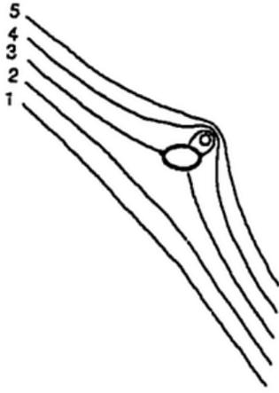
Fig. 2: The uniform flow obtained when a vortex at the position (2.236,0.758). The streamlines labeled 1, 2, 3, 4 and 5, correspond to  $\Psi = -1.0, -0.5, 0.0, 0.5$  and  $1.0$ , respectively.
