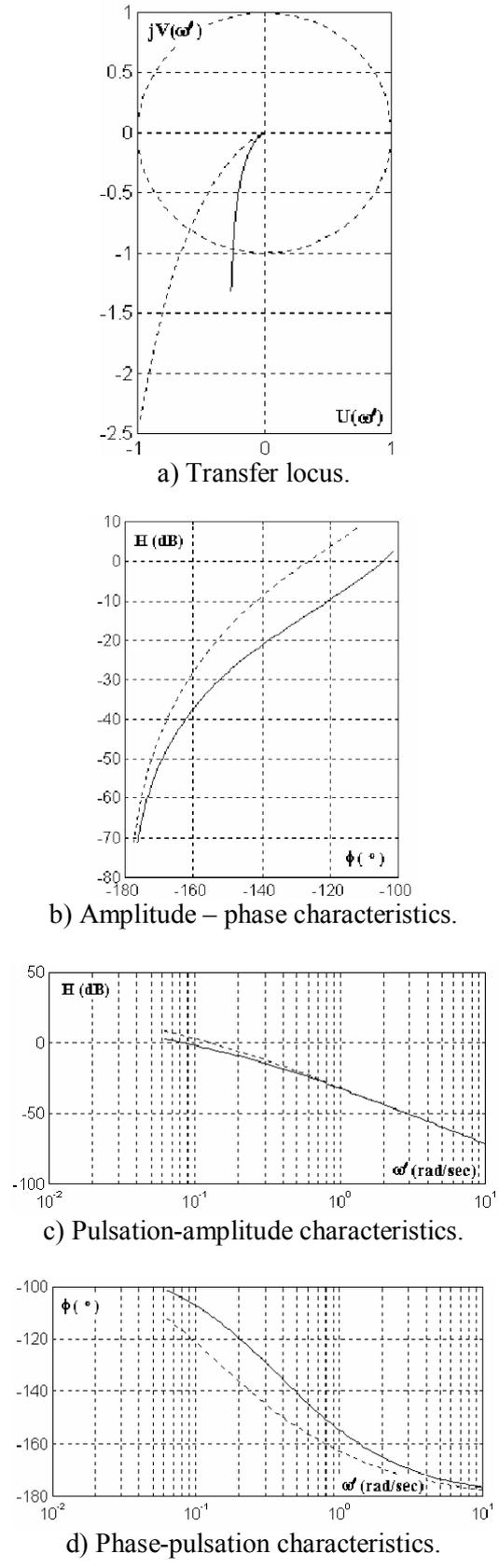
Fig.3. Graphics dependences corresponding to the cases  $R'_r=5,5 \Omega$  (continuous line) and  $R'_r=4,5 \Omega$  (dot line).
