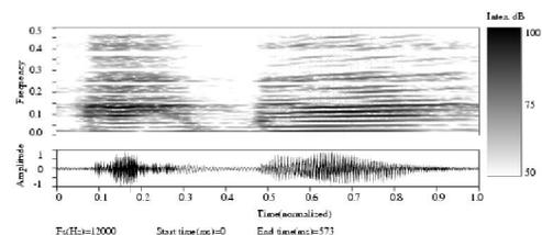
**Fig. 8 Narrowband spectrogram of processed /aba/ with CF=0.7**
