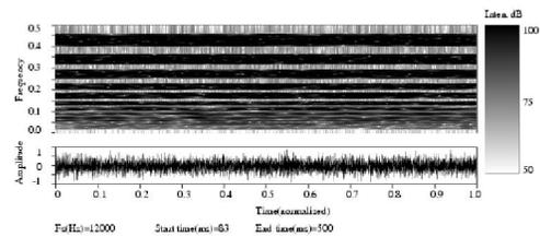
**Fig. 6 Narrowband spectrogram of processed broadband noise with CF=0.5**
