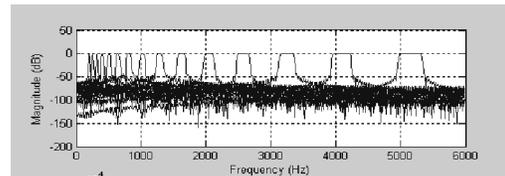
**Fig. 2 Frequency responses of the 15 frequency bands of the synthesis filter bank to accomplish frequency compression of 0.3**
