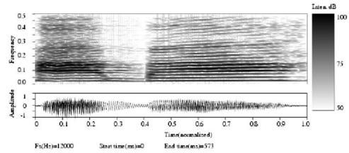
**Fig. 4 Narrowband spectrogram of unprocessed VCV syllable /aba/**
