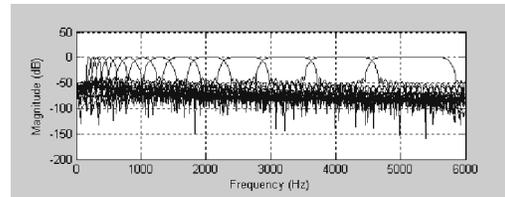
**Fig. 1 Frequency responses of the 15 frequency bands of the analysis filter bank**
