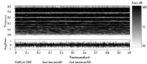
**Fig. 5 Narrowband spectrogram of processed broadband noise with CF=0.7**
