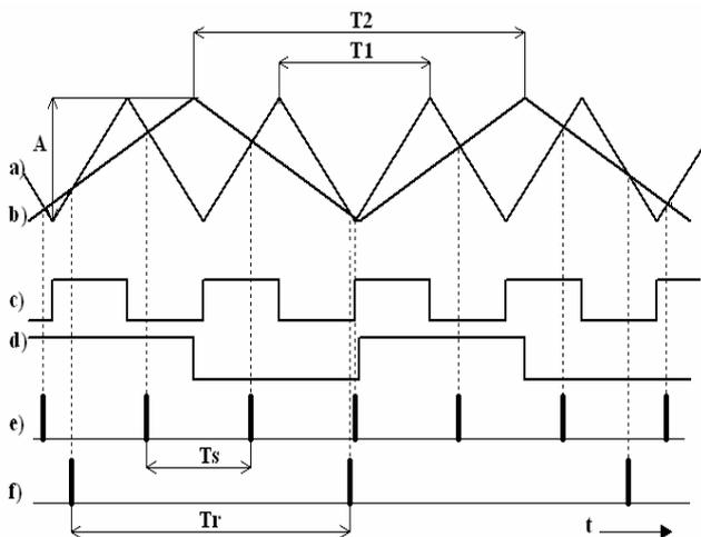
Fig. 7. Coincidence mixer time diagram. a) input signal with frequency  $f_1$  (period  $T_1$ ), b) input signal with frequency  $f_2$  (period  $T_2$ ), c) derivation of signal a), d) derivation of signal b), e) output pulses with frequency  $f_S = f_1 + f_2$  (period  $T_S$ ) f) output pulses with frequency  $f_R = \text{abs}(f_1 - f_2)$  (period  $T_R$ ).
