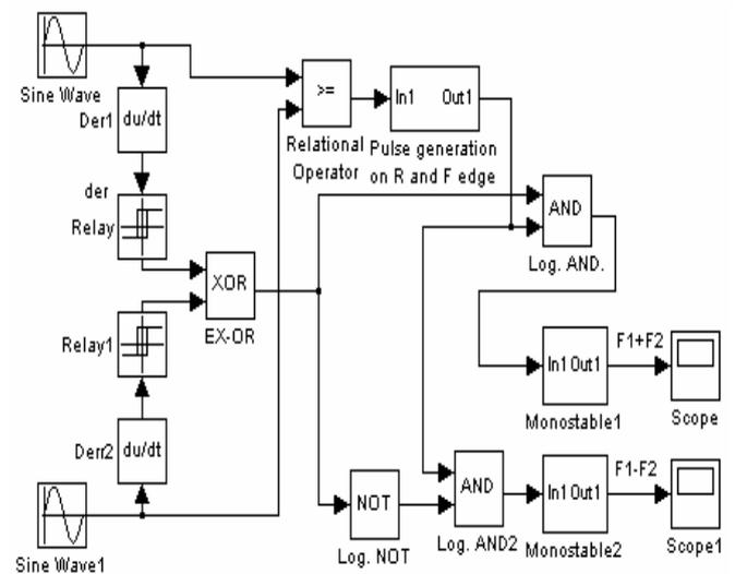
Fig. 11. Block diagram of coincidence mixer for Matlab simulation. The mixer has 2 output  $F_1 + F_2$  and absolute value of  $F_1 - F_2$ . The Relay blocks are used as a converter to digital signal level.
