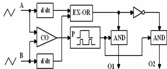
Fig. 10. Block diagram of coincidence mixer. A, B - input signals, d/dt - derivation block, CO - comparator, P - pulse block which generate pulse on rising and falling edge, EX-OR - exclusive-or gate, AND - logical and gate, O1 - output with sum of input frequencies, O2 - output with difference of input frequencies.
