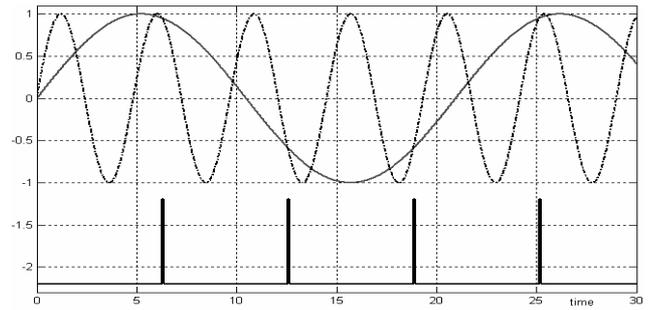
Fig. 9. Coincidence mixer - time diagram (Simulation result). Input signals (top) and output pulses (bottom). Frequency of output pulses is difference of input frequencies.
