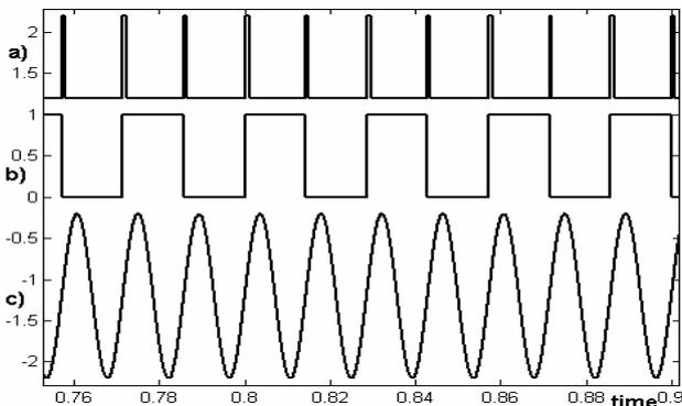
Fig. 12. The sine signal recovery. a) Mixer pulse output, b) Square wave pulses, c) Sine signal (PLL output).
