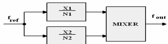
Fig. 5. Block diagram of synthesizer part
