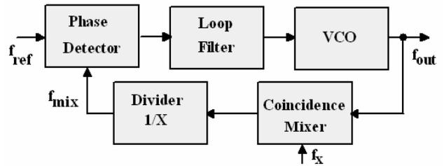
Fig. 14. The Phase-Locked-Loop with coincidence mixer and divider placed in feedback.
