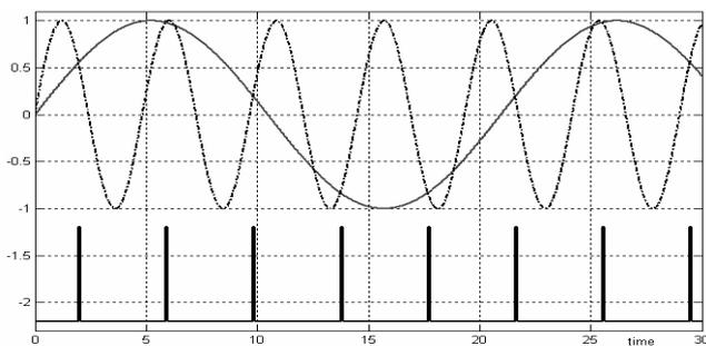
Fig. 8. Coincidence mixer - time diagram (Simulation result). Input signals (top) and output pulses (bottom). Frequency of output pulses is sum of input frequencies.
