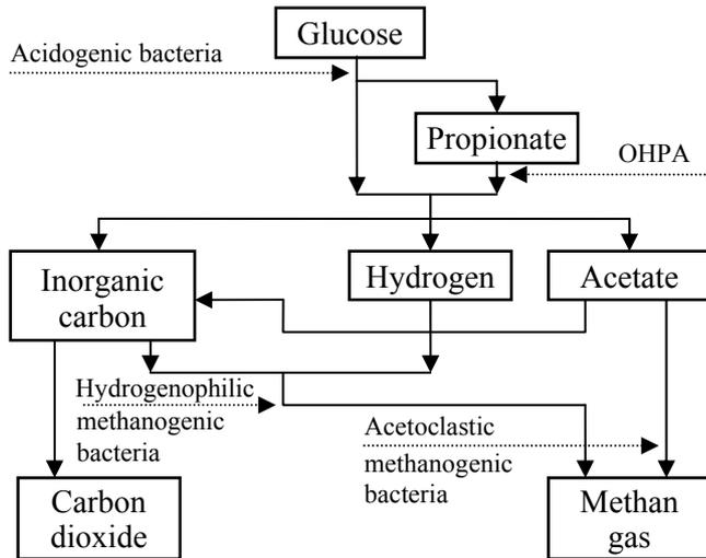
Fig.1. A schematic view of anaerobic digestion process
