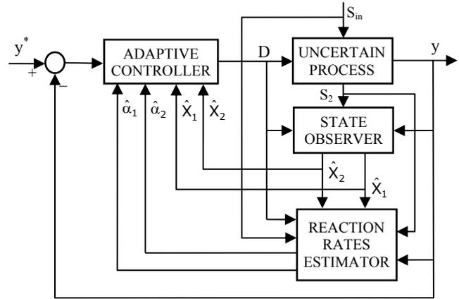
Fig.2. The structure of the adaptive system
