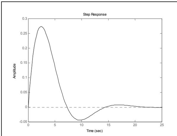
Fig. 4 Step response of  $H_2(s)$
