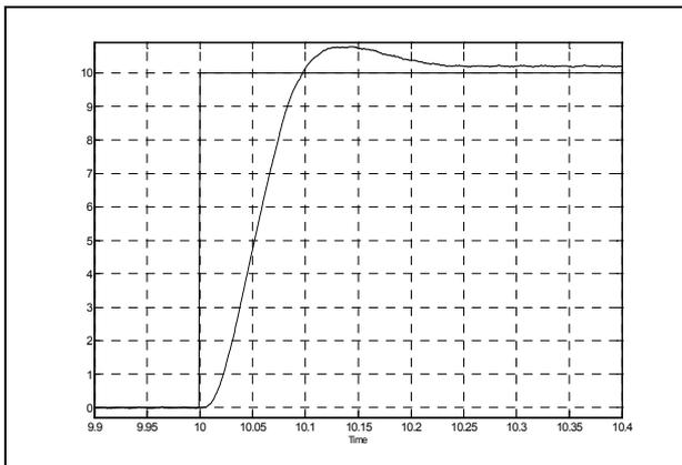
Fig. 6 Step response of the closed-loop system with controller gain  $K_c=0.2$
