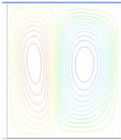
Fig.8 Numerical streamlines for  $\delta=0.4$  ( $Ra=2 \cdot 10^5$ )
