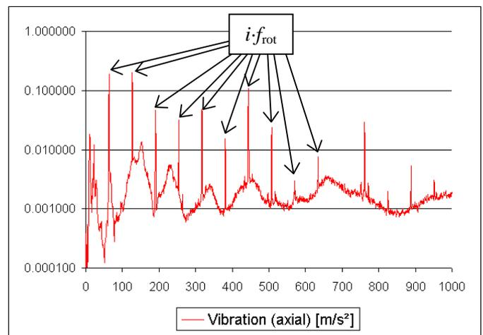
**Fig. 3** Vibration spectrum of a ECM drive running at 3800RPM: Vibration is excited by radial force at multiples of the rotation frequency.
