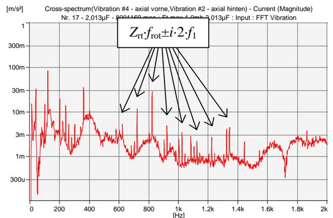
**Fig. 2** Vibration spectrum caused by radial force in a single-phase induction motor
