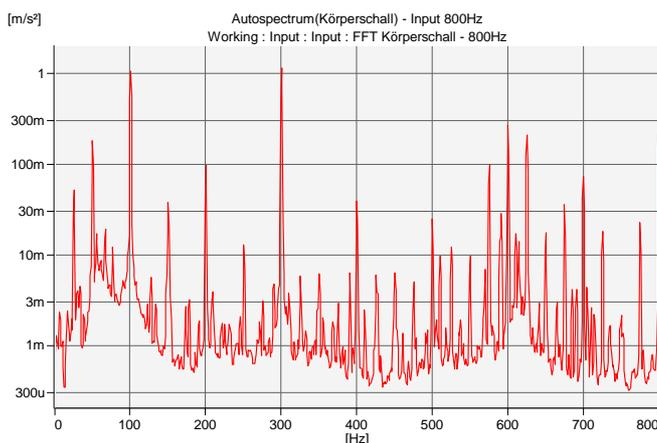
**Fig. 1** Vibration spectrum showing strong peaks at multiples of 100Hz caused by magnetostriction
