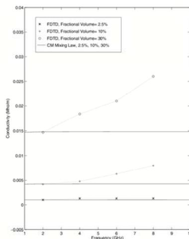
Figure 5: Comparison of FDTD results for the imaginary part of the dielectric constant with the CM mixing law.
