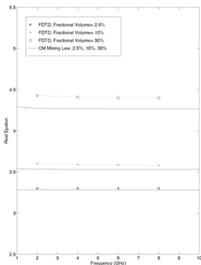
Figure 4: Comparison of FDTD results for the real part of the dielectric constant with the CM mixing law
