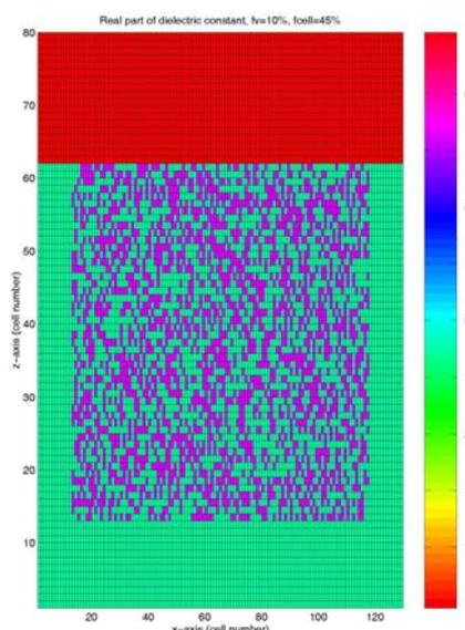
Figure 2: A two-dimensional cut through the FDTD domain.
