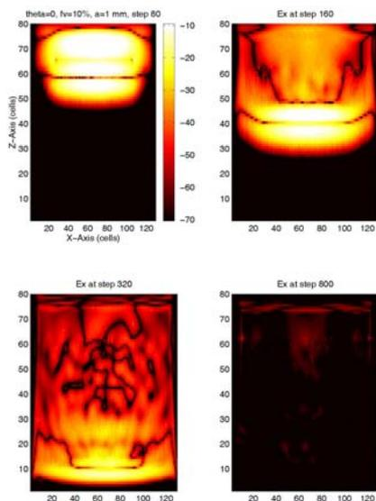
Figure 3: Wave propagation in the FDTD domain at several time instants
