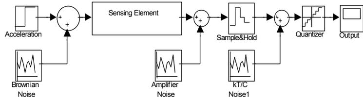
Figure 2: Noise model of MEMS accelerometer [5]
