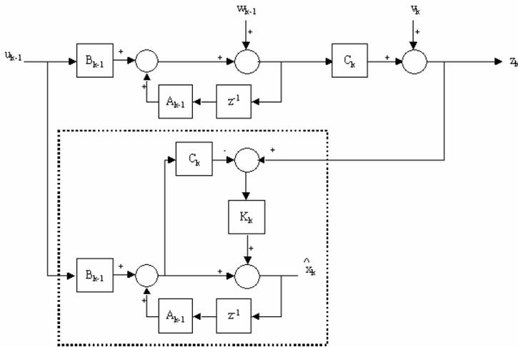
Figure 3: Linear discrete system with Kalman filter [10]
