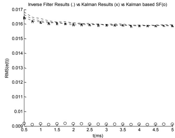
Figure 9: Measurement error using Inverse Filters vs individual KFs vs KF based Sensor Fusion
