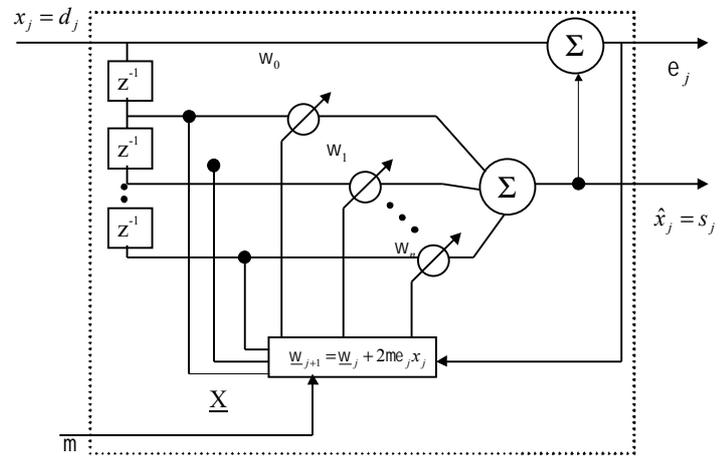
Figure 4: LMS Adaptive Filter [9]
