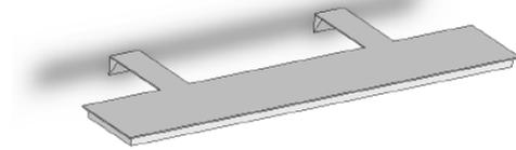
Figure 6: Double Cantilever Beam Piezoresistive Accelerometer [4]
