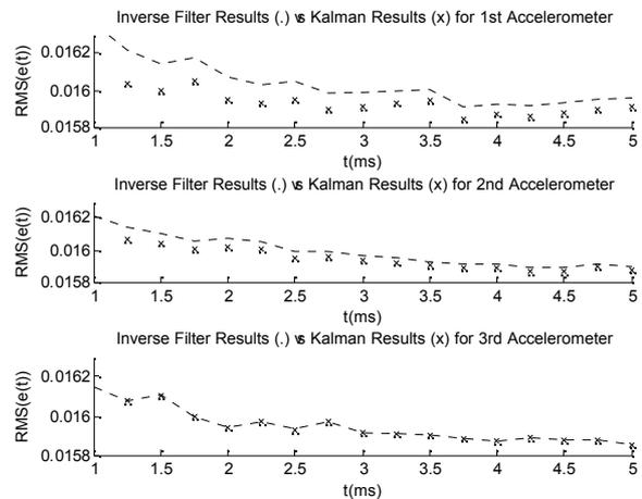
Figure 8: (a) Inverse Filter vs Kalman Filter for 1<sup>st</sup> 1-DOF Accelerometer, (b) Inverse Filter vs Kalman Filter for 2<sup>nd</sup> 1-DOF Accelerometer, (c) Inverse Filter vs Kalman Filter for 6-DOF Accelerometer
