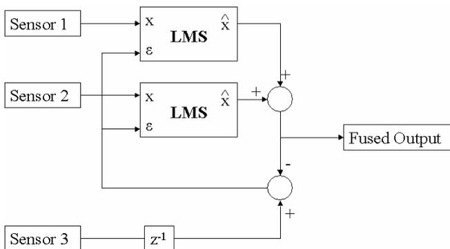
Figure 5: LMS Based Sensor Fusion Diagram
