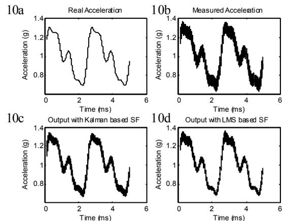
Figure 10: (a) Noiseless acceleration output, (b) Noisy acceleration output, (c) output which is fused with Kalman based Sensor Fusion, (d) output which is fused with LMS based Sensor Fusion.
