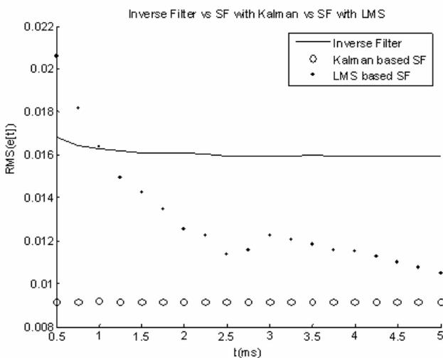
Figure 11: Comparison of errors obtained in inverse filter, SF with Kalman and SF and LMS
