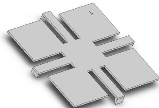
Figure 7: Double Cantilever Beam Piezoresistive Accelerometer [8]
