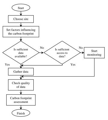
Fig. 6 Carbon footprint flow chart.
