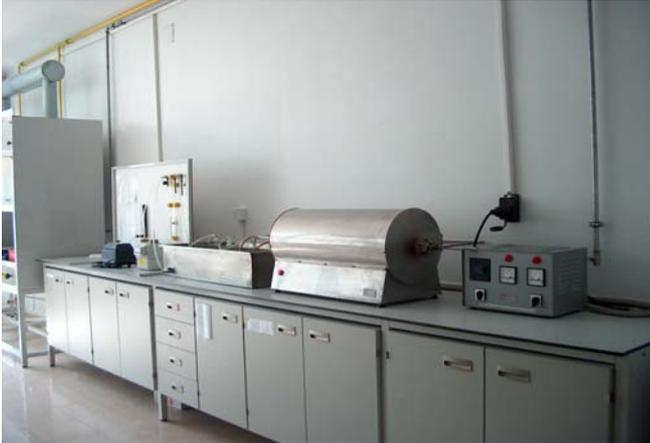
Figure 1 Laboratory scale tube incinerator
