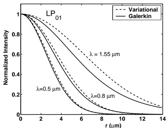
Fig. 5: Normalized intensity distribution of the  $LP_{01}$  mode of the TEC-fiber for different wavelengths. The radius of the expanded core of the fiber is  $A = 8\mu m$ .
