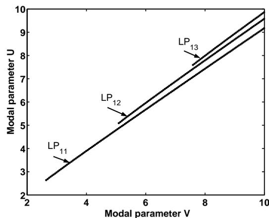
Fig. 2: Plots of the modal parameter  $U$  as a function of the normalized frequency  $V$  for the first three  $LP_{1l}$ -modes.
