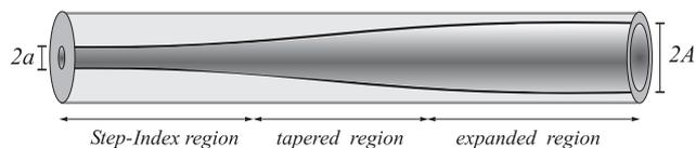
Fig. 1: Schematic illustration of a thermally expanded core fiber.
