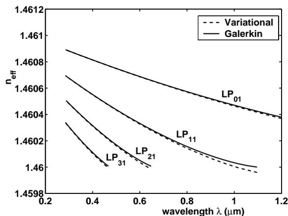
Fig. 4: Effective indices  $n_{eff}$  of the first three  $LP_{ml}$ -modes as a function of the wavelength.
