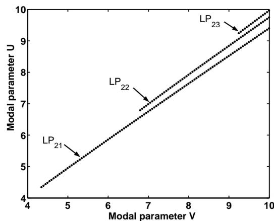
Fig. 3: Plots of the modal parameter  $U$  as a function of the normalized frequency  $V$  for the first three  $LP_{2l}$ -modes.
