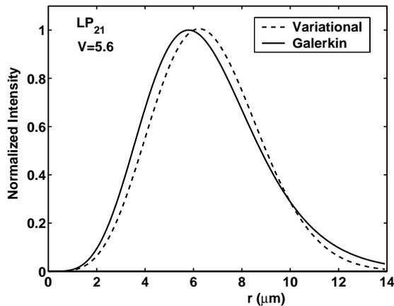
Fig. 7: Normalized intensity distribution of the  $LP_{21}$  mode of the TEC-fiber for  $V = 5.6$ . The radius of the expanded core of the fiber is  $A = 8\mu m$ .
