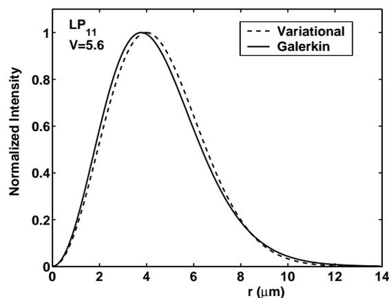
Fig. 6: Normalized intensity distribution of the  $LP_{11}$  mode of the TEC-fiber for  $V = 5.6$ . The radius of the expanded core of the fiber is  $A = 8\mu m$ .
