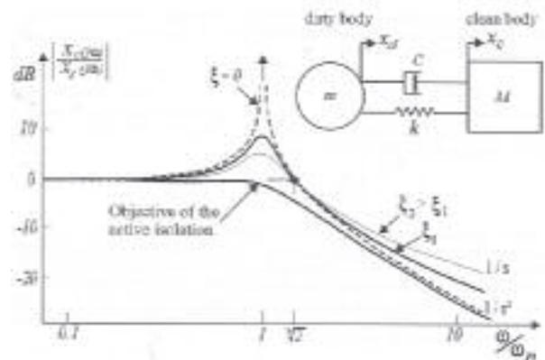
Fig. 2 FRF of passive isolator transmissibility for different values of the damping [4]
