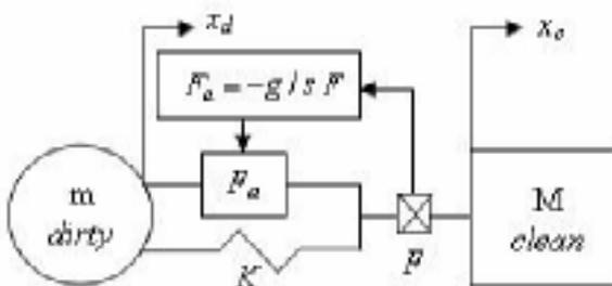
Fig. 4 Force feedback isolator [4]
