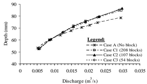
Fig. 3: Stage-discharge curves of different block densities for fixed bed
