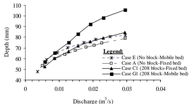
Fig. 5: Stage-discharge relationships between fixed bed and mobile bed cases
