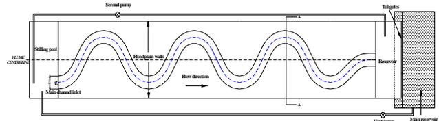
Fig. 1: Experimental flume plan
