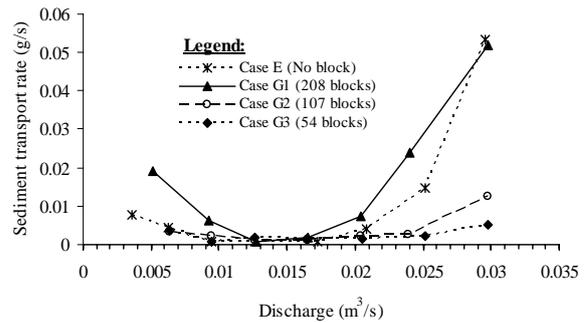
Fig. 7: Discharge and sediment transport relationship for mobile bed channel cases
