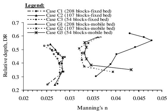
Fig. 6: Manning's n of different block densities for fixed bed and mobile bed
