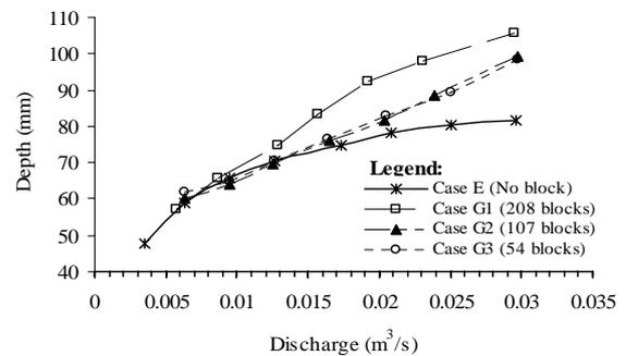
Fig. 4: Stage-discharge curves of different block densities for mobile bed
