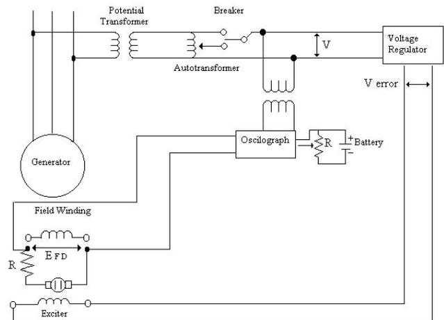
Fig 6. Method of the variable autotransformer directly feeder from the generating unit terminals.
