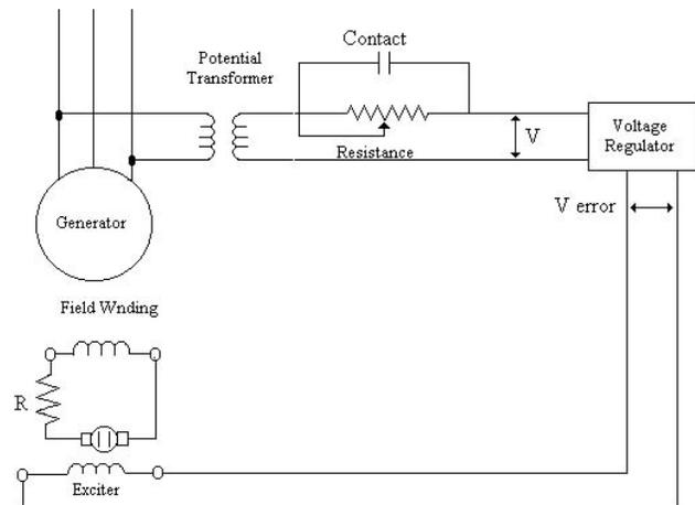
Fig 8. Test method using a variable resistance connected in series with the secondary of the potential transformer.
