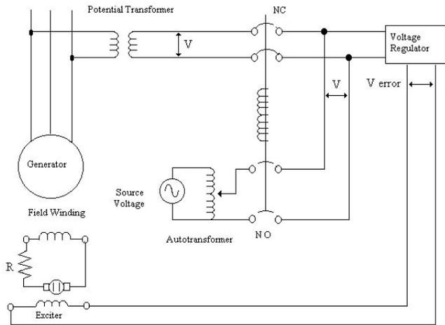
Fig 7. Test method arranging the variable autotransformer feeder from an external voltage source.
