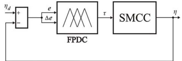
Fig. 2. A structure of the fuzzy controller
