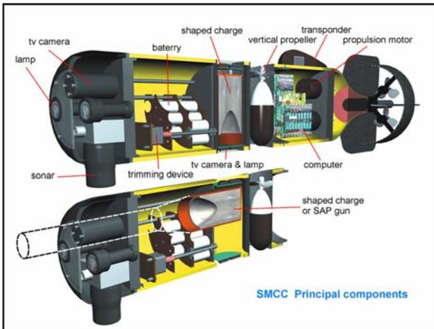
Fig. 1. Main parts of the SMCC
