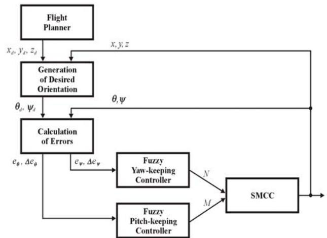
Fig. 4. A block-diagram of the control system
