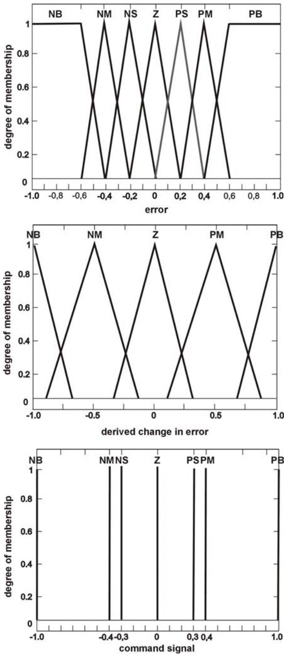
Fig. 3. Fuzzifier membership functions of error signal  $e$ , derived change in error  $\Delta e$  and command signal  $\tau$
