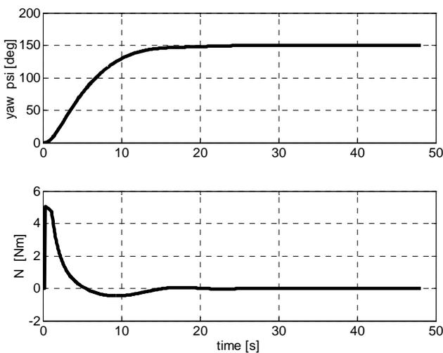
Fig. 6. Time histories of yaw  $\psi$  and moment about vertical axis  $N$  for surge velocity  $u = 1.5$  m/s
