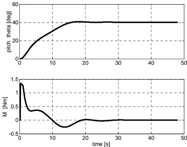
Fig. 5. Time histories of pitch  $\theta$  and moment about transversal axis  $M$  for surge velocity  $u = 1.5$  m/s
