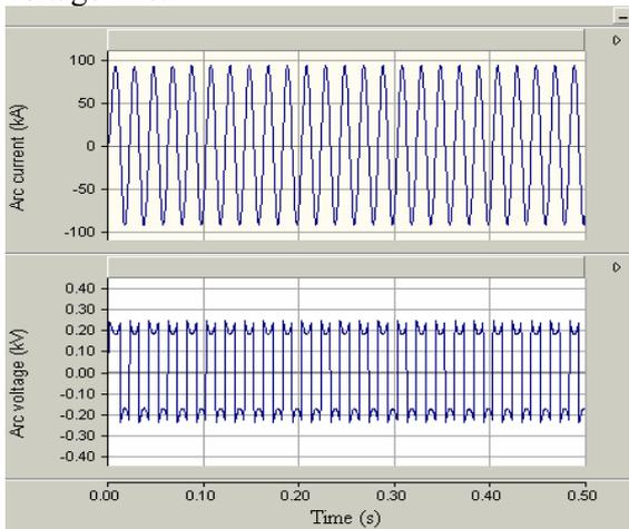
Fig. 4. The variation of arc current and voltage according to relations (29) and (30).
