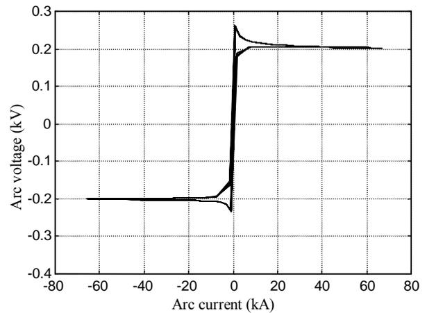
Fig. 7. The characteristic current-voltage of the electric arc for phase 1, obtained by simulation.
