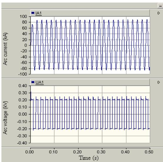
Fig. 6. The variation of the arc current, voltage and resistance, for  $U_l = 520 V$ .
