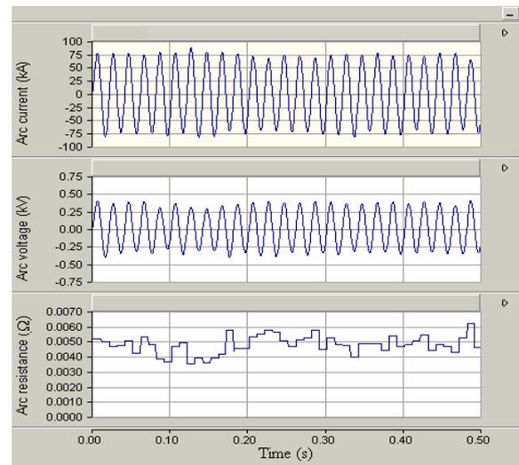
Fig. 2. The variation of the arc current, voltage and resistance according to relation (3).
