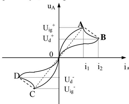
Fig. 3. The real and line characteristic of the electric arc.
