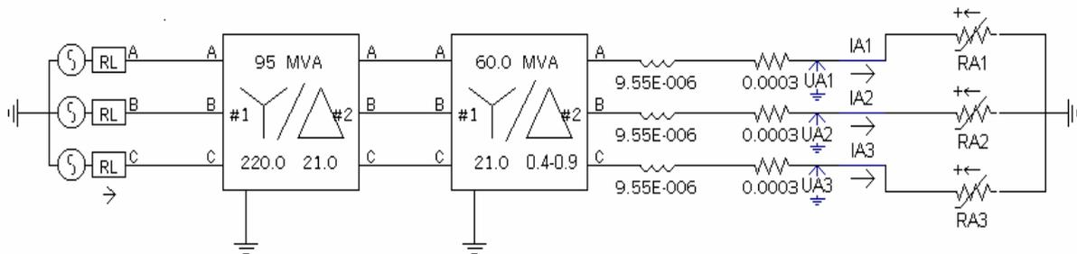
Fig. 1. Diagram of the electric installation of the arc furnace
