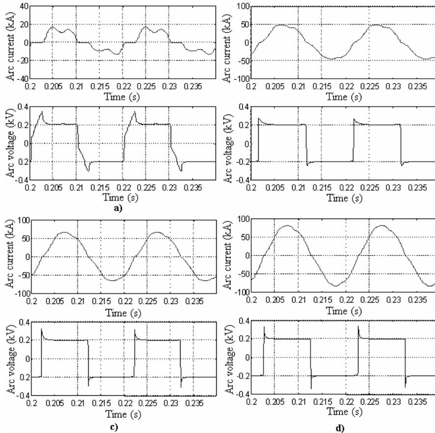
Fig. 5. The variation of the arc current and voltage for various values of the voltage given by the secondary of the furnace transformer a) 380V; b) 450 V; c) 520 V; d) 600V.
