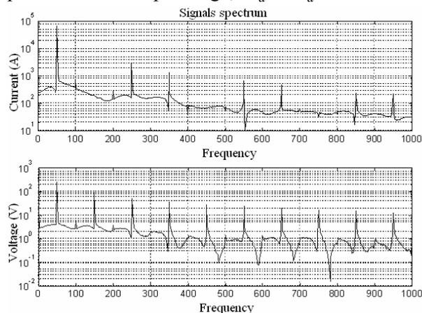
Fig. 8. The spectral characteristic of the electric arc current and voltage
