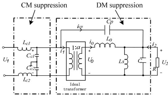
Fig.11 Equivalent DM and CM circuits of IFT
