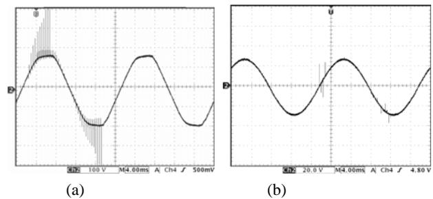
Fig.13 Input and output voltages of IFT (a) Input voltage (b) Output voltage
