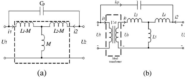
Fig.3 Analytic circuit (a) T-circuit (b) analytic circuit with ideal transformer
