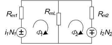
Fig2 Equivalent magnetic circuit
