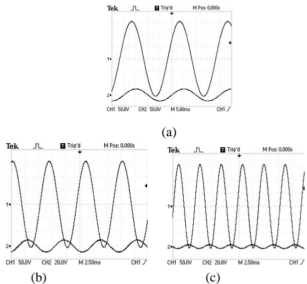
Fig 8 Experiment waveforms in different frequency with rated loads (a) 50Hz (b) 150Hz (c) 250Hz
