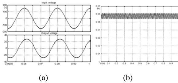
Fig.6 Simulation waveform (50Hz input voltage with rated load) (a) input and output voltage waveforms (b)  $L_S(t)$
