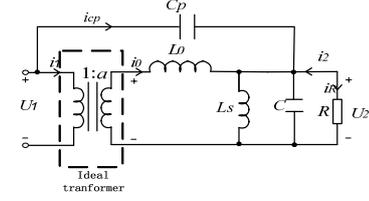
Fig.4 Equivalent circuit of the DM part of IFT
