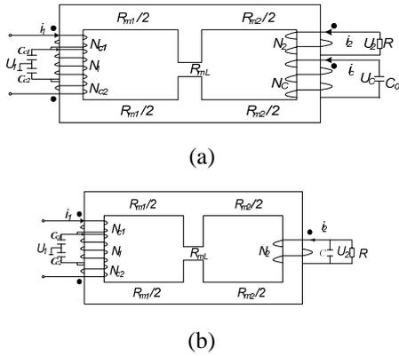
Fig.1 Structure & Equivalent structure of IFT (a) Structure of IFT (b) Equivalent structure of IFT
