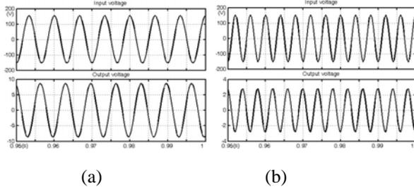
Fig.7 Simulation waveform of high frequency input and output voltage (a) 150Hz (b) 250Hz
