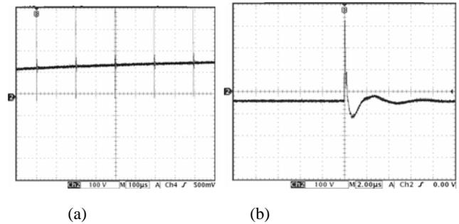
Fig.12 Output waveform of NS64000-4A (a)Bursts' waveform (b) Single burst waveform
