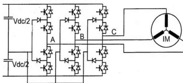
Fig-1 Three-level voltage source inverter feeding an induction motor
