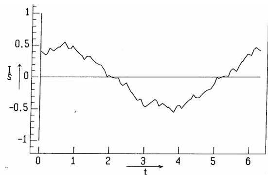
Fig.3 Space vector and phase stator steady-state current
