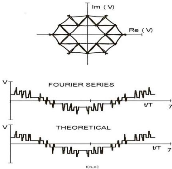
Fig.4 Space vector of the stator voltage vector and its phase waveform (theoretical and from Fourier expansion)
