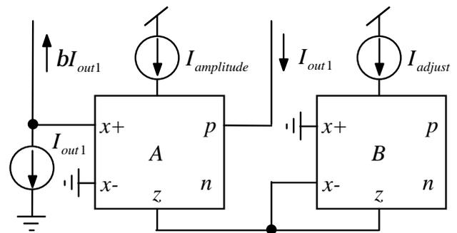
Fig. 2: Proposed circuit for automatic gain control.
