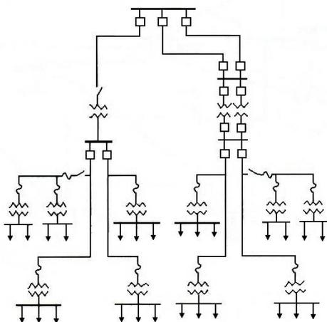
Figure 2: A simple radial distribution system.
