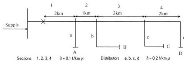
Figure 3: A typical radial distribution system.
