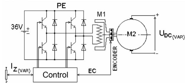
Fig. 7. Diagram of connection of the tested machine model to the electronic power converter for determination of the external characteristics of the machine, where: 36V – power supply battery; PE – electronic power converter; M1 – tested machine model; M2 – driving motor of the tested assembly; EC – signal synchronizing the controllable polarizable current source of the converter;  $I_z$  – setting signal of the current source of the converter.
