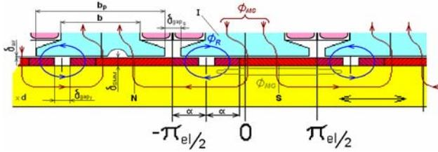
Fig. 2. Distribution of the field magnet flux  $\Phi_{MG}$  into the component fluxes  $\Phi_{MS}$  and  $\Phi_R$  for a given angle  $\alpha$  of the field magnet shift in relation to the stator teeth.
