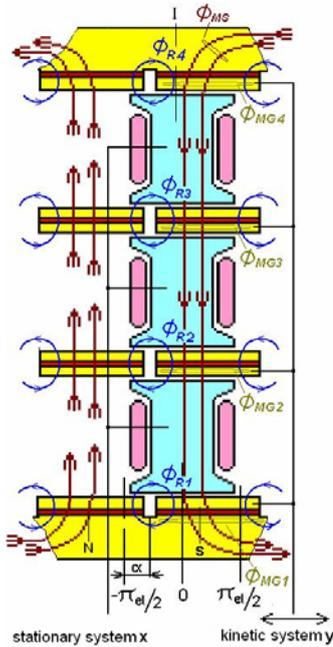
Fig. 4. Distribution of magnetic fluxes in a pole of a machine as in Fig. 1b during rotation of the field magnet by angle  $\alpha$  in relation to a stator tooth for the idle run state.
