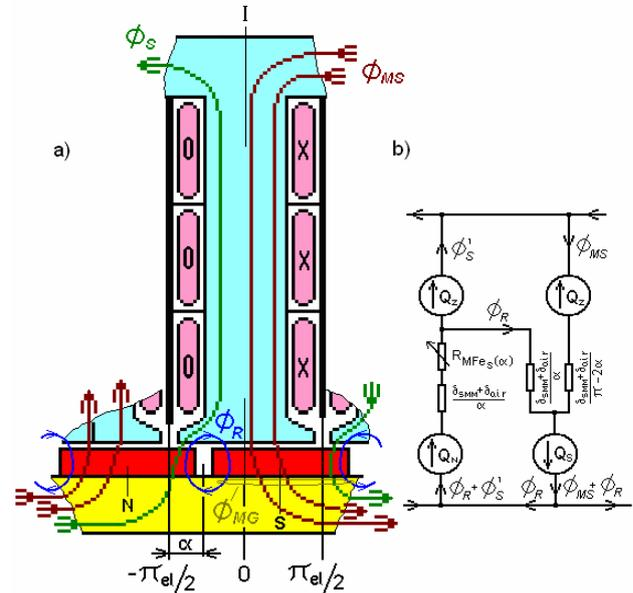
Fig. 5a. View of a pole of a conventional machine for the loaded state with marked distribution of magnetic fluxes for the assumed direction of the winding current and the field magnet rotation angle  $\alpha$ .
