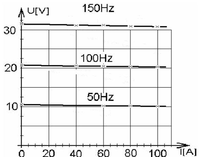
Fig. 10. External characteristics of the machine at loading with the electronic power converter with forced waveform of the current compatible with the internal voltage of the machine, for the frequencies 50, 100 and 150Hz (shaft speeds 167, 333 and 500rpm, respectively).
