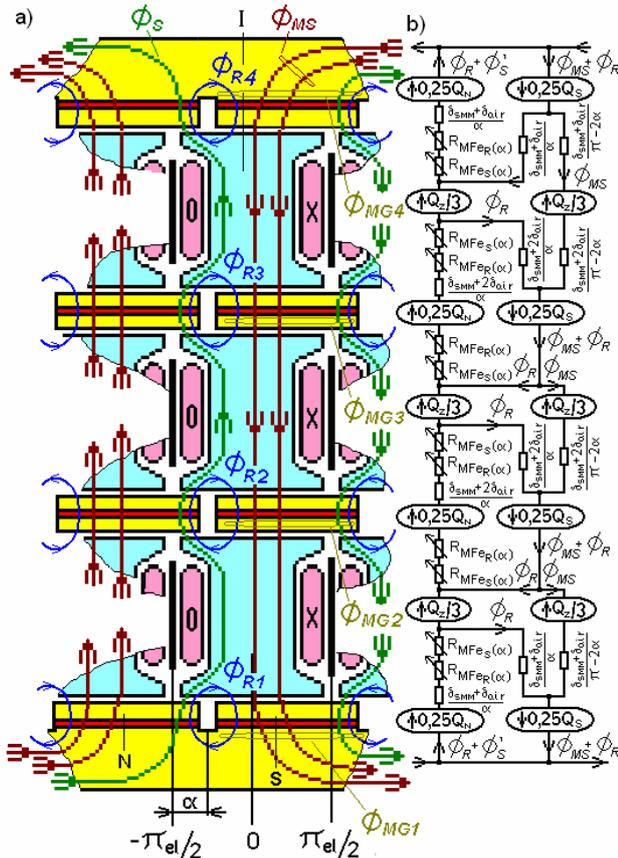
Fig. 6a. View of a pole of the machine model constructed according to the slot cutting conception for the loaded state with marked distribution of magnetic fluxes for the assumed direction of the winding current and the field magnet rotation angle  $\alpha$ .
