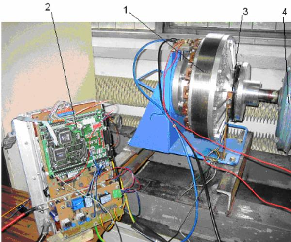
Fig. 8. Assembled model of the machine (1) constructed according to the slot cutting conception on the test stand together with the electronic power converter (2), the embedded encoder (3) and the driving machine (4).
