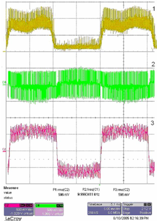
Fig. 9. Basic waveforms of current and voltage for generator operation of the machine for 50Hz, where:
