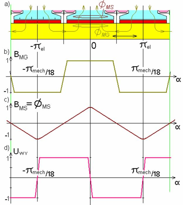
Fig. 3. Basic waveforms of magnetic fluxes in the reactive structures of machines as in Fig. 1a and b during movement of the field magnet poles in relation to the stator, where:
