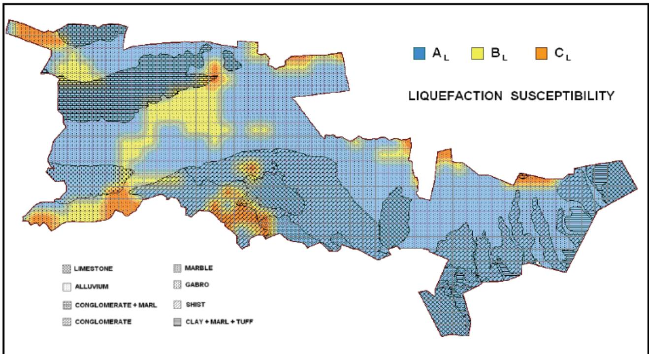
Fig.5 Liquefaction susceptibility map prepared by ABS Consulting
