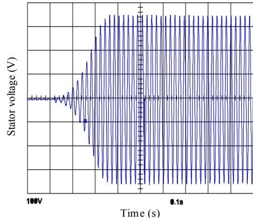
Fig. 5. Measured stator voltage during the self-excitation process at 1500 rpm and 90 $\mu$ F.
