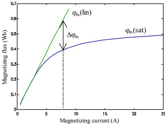
Fig. 2. Magnetization curve of the studied induction machine.
