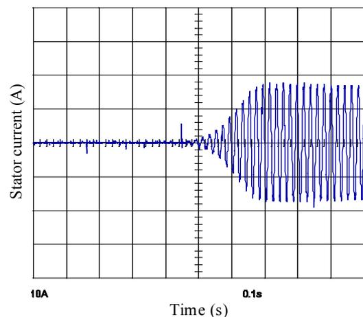
Fig. 7. Measured stator current during self-excitation process at 1500 rpm and 90 $\mu$ F.
