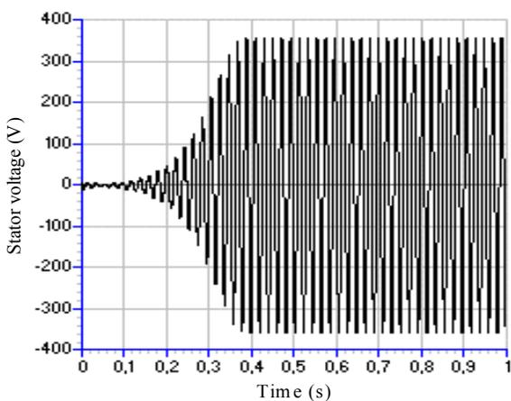
Fig. 4. Computed stator voltage during the self-excitation process at 1500 rpm and 90 $\mu$ F.
