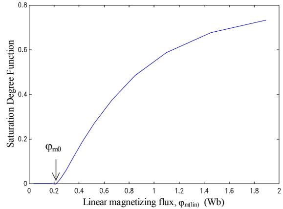
Fig. 3. Variation of the SDF as a function of the linear magnetizing flux.
