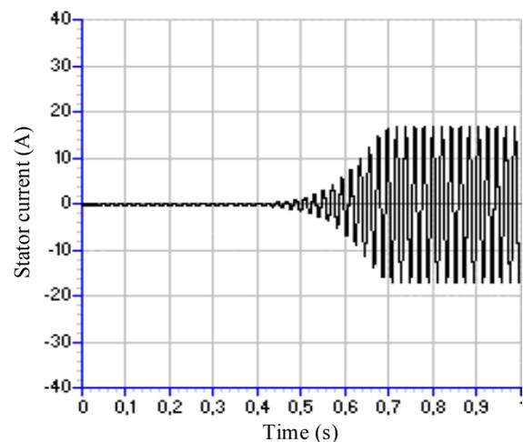
Fig. 6. Computed stator current during self-excitation process at 1500 rpm and 90 $\mu$ F.
