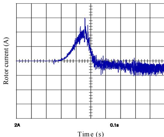
Fig. 9. Measured rotor current during self excitation process at 1500 rpm and  $90\mu\text{F}$ .
