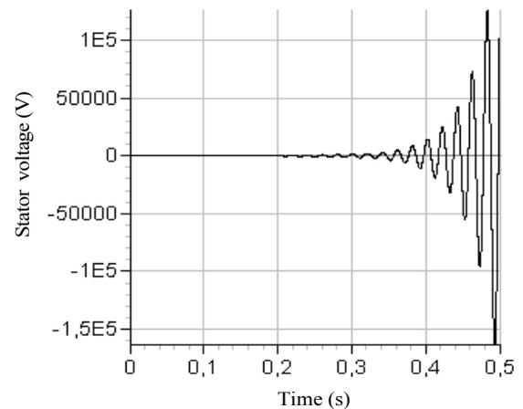
Fig. 1. Computed stator voltage during the self-excitation process when the saturation effect is neglected.
