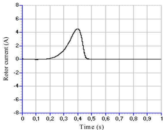
Fig. 8. Computed rotor current during self excitation process at 1500 rpm and  $90\mu\text{F}$ .
