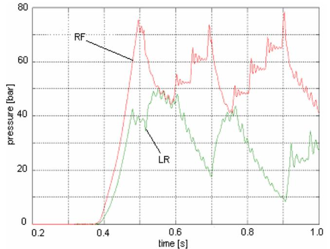
Figure 1 – Example of the problems related to a not sufficient pump volume displacement during ABS modulation
