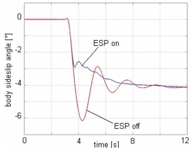
Figure 11 – Time history of body sideslip angle with and without ESP for the same vehicle; step steer in the condition of a low friction coefficient between tires and ground
