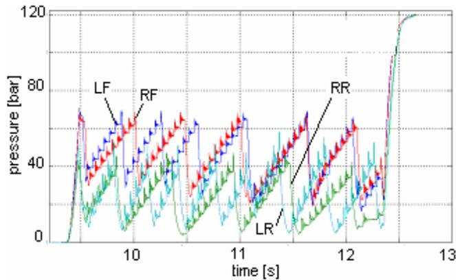
Figure 3 – Example of the implementation of the conceived ABS algorithm on a new generation commercial ESP unit (its pump has a larger flow rate)
