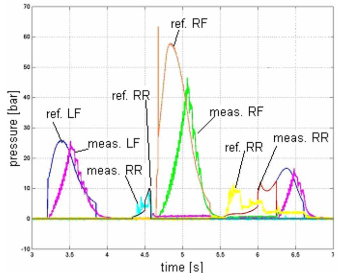
Figure 10 – Time history of reference ('ref.') and measured ('meas.') calipers pressures during an extreme double step steer maneuver
