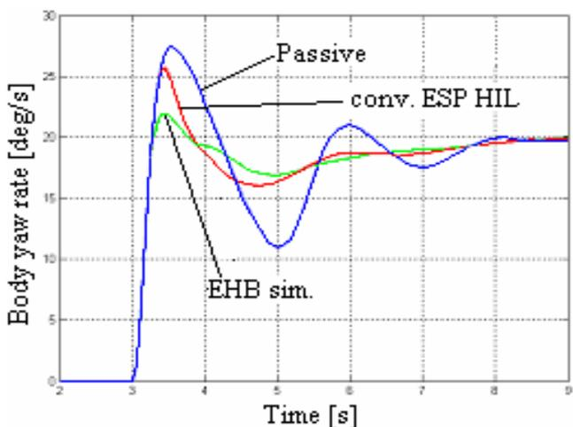
Figure 13 – Time history of body yaw rate during an extreme step steer maneuver (high friction coefficient between tires and ground); comparison between a passive vehicle ('Passive'), a vehicle with a conventional ESP hydraulic unit ('conv. ESP HIL') and a vehicle with an EHB ('EHB sim.') unit
