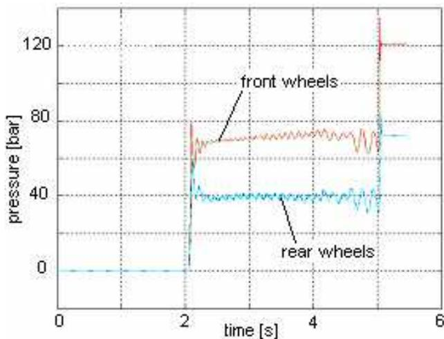
Figure 4 – Example of improvement of the ABS performance related to the adoption of an EHB hydraulic unit [3]
