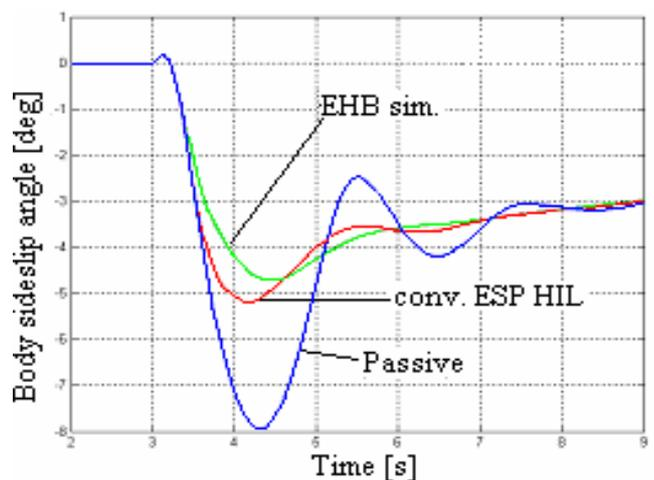
Figure 14 – Time history of body sideslip angle during an extreme step steer maneuver (the same maneuver of Figure 13); comparison between a passive vehicle ('Passive'), a vehicle with a conventional ESP hydraulic unit ('conv. ESP HIL') and a vehicle with an EHB ('EHB sim.') unit
