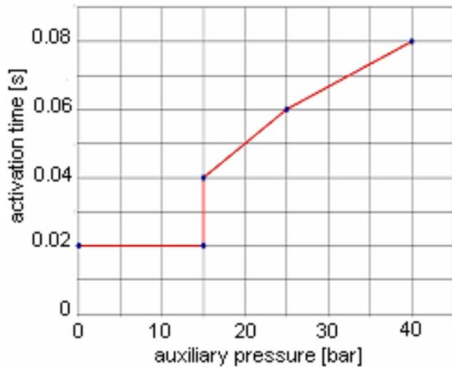
Figure 5 – Minimum duration of pump intervention as a function of  $p_{auxiliary}$
