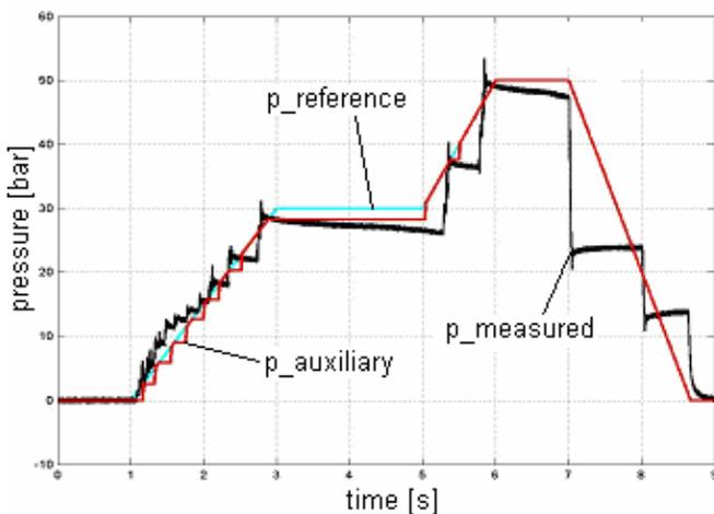
Figure 6 – Example of test to verify the performance of the actuation algorithm
