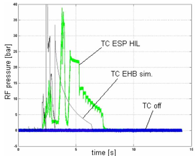
Figure 8 – Time history of low adherence caliper pressure during a start-up maneuver in split- $\mu$  conditions
