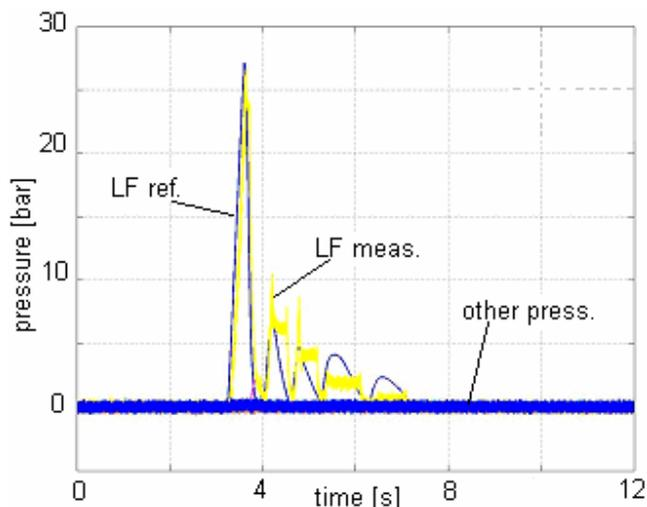
Figure 12 – Time history of reference ('ref.') and measured ('meas.') Left Front ('LF') and other ('other press.') calipers pressures during the same maneuver of Figure 11
