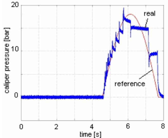
Figure 7 – Example of test to verify the performance of the actuation algorithm: comparison between reference and measured pressures
