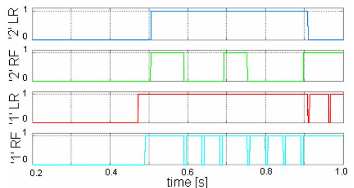
Figure 2 – Modulation of valves '1' and '2' (Figure 1) for Right Front (RF) and Left Rear (LR) wheels during the same brake maneuver of Figure 1
