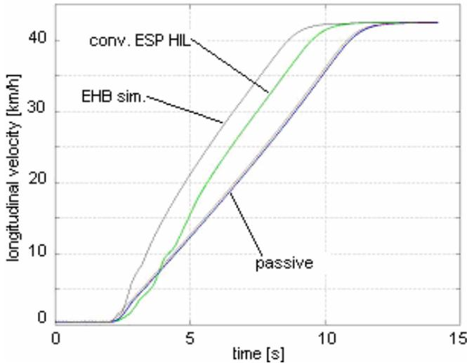
Figure 9 – The effect of the performance of the ESP hydraulic unit from the point of view of vehicle longitudinal speed
