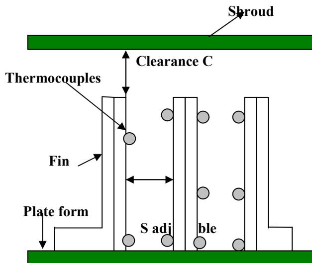
Fig. 2 (a) Experimental set up (schematic)
