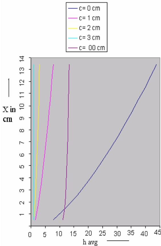
Fig 5 Variation in “h” along fin length for different clearance
