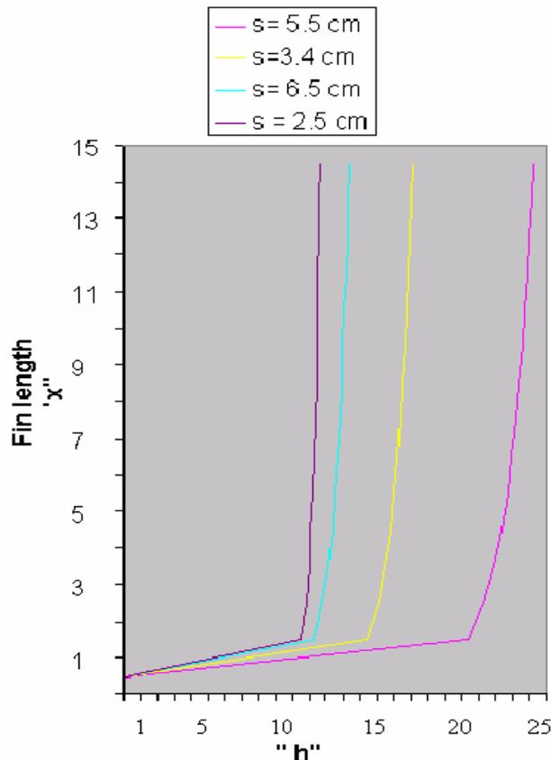
Fig. 4 Variation in “h” along fin length for different Inter-fin Spacing (For  $C = \infty$ )
