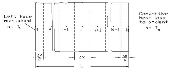
Figure 2: Grid for a slab of width L initially at temperature of  $T_i$
