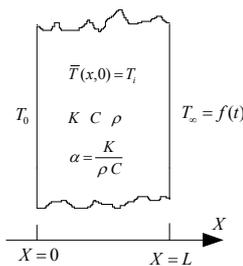
Figure 1: schematic representation of steel slab
