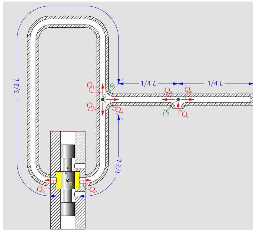
Figure 1: Geometry of the hydraulic wave converter.
