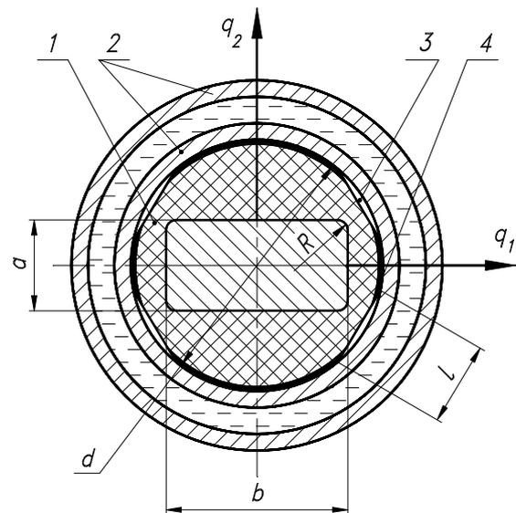
Fig. 1. Scheme of the regulation of heat transfer in the round mould.
