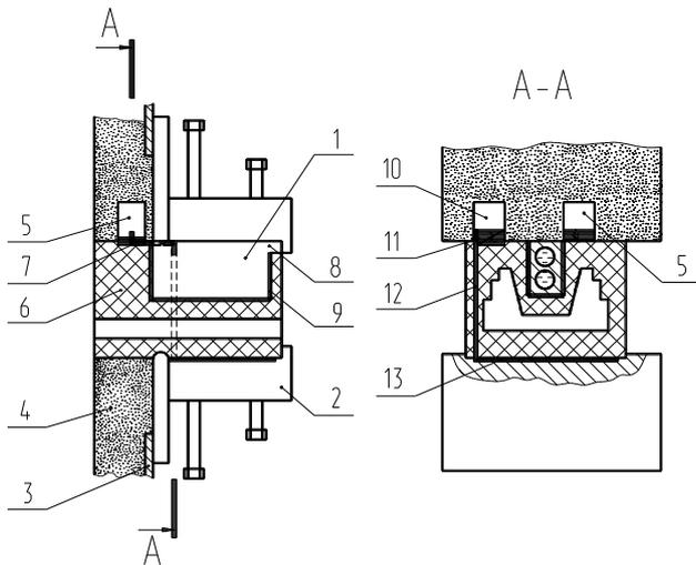
Fig. 3. Scheme of the mould with fusible interlayer: 1 - upper water cooled jacket; 2 - lower water cooled jacket; 3 - crucible wall; 4 - crucible lining; 5 and 10 - tin cylinders; 6 - graphite sleeve; 7, 11 and 12 - gates; 8 - overflow; 9 - upper interlayer; 13 - lower interlayer.
