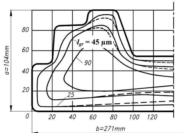
Fig. 4. Exchange of the length of graphite inclusions in the microstructure of grey iron castings produced in the ordinary mould (continuous line) and in the mould with fusible interlayer (dotted line).
