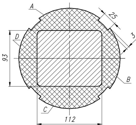
Fig. 2. Cross-sections of graphite sleeve and casting.
