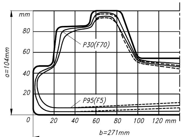
Fig. 5. Quantity of pearlite in the microstructure of castings of grey cast iron produced in the ordinary mould (continuous line) and in the mould with fusible interlayer (dotted line).
