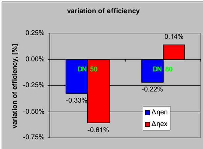
Fig. 5: Influence of the connection pipeline's tube diameter on the energetic and exergetic total efficiency (nominal diameter 65 mm)
