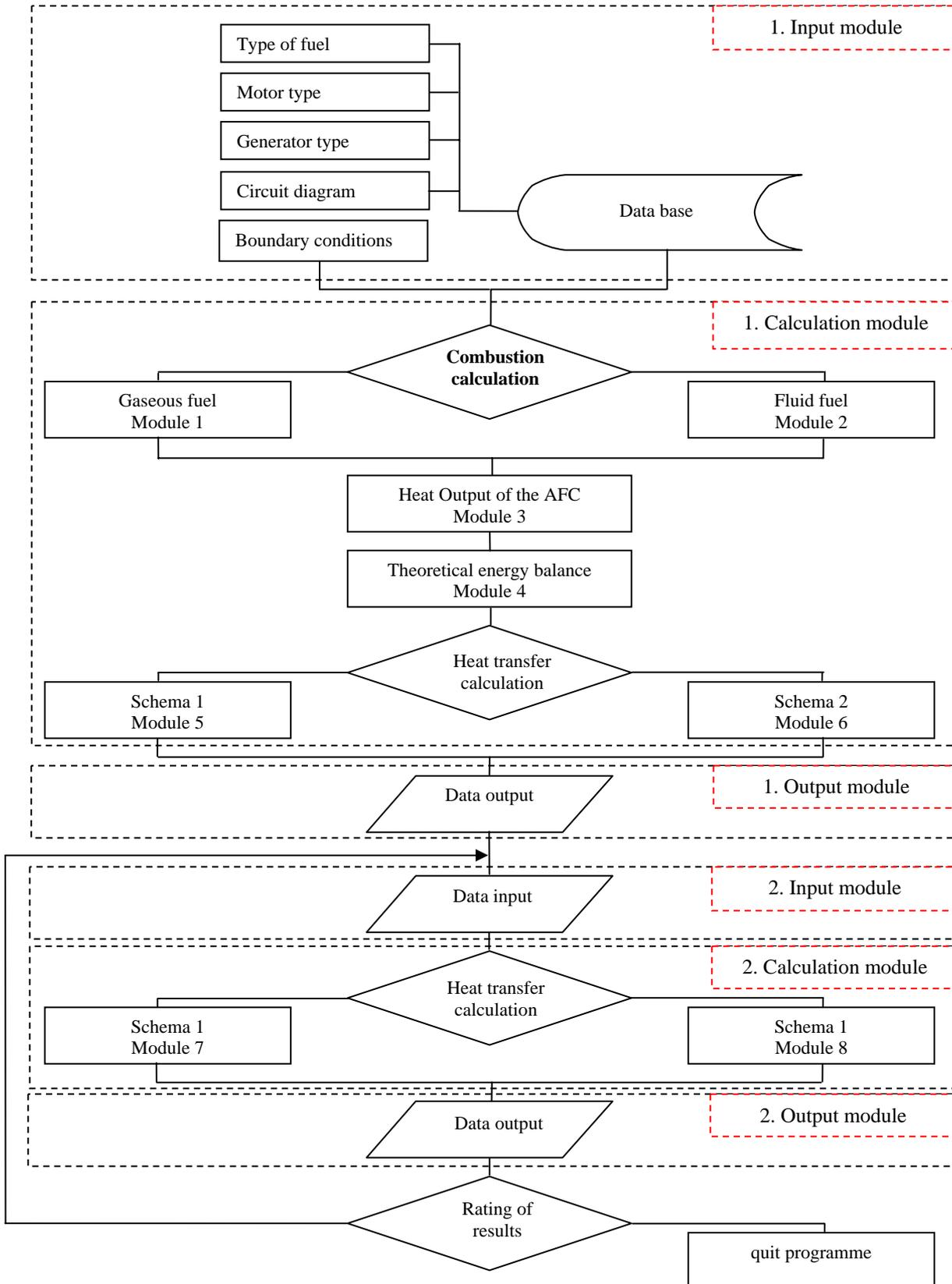
Fig. 4: Algorithm for calculation and modelling of Total Energy Units
