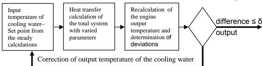
Fig. 3: Method of iteration to determine the quasi-steady operating conditions
