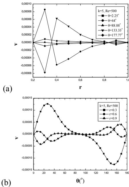
Fig. 7. (a) Variation of meridional component of velocity with radial distance at  $\theta = 2.25^\circ, 44^\circ, 88.88^\circ, 133.33^\circ, 177.77^\circ$  for  $Re = 500$  and  $k = 5$ ; (b) Variation of meridional component of velocity with meridional coordinate  $\theta$  at  $r = 0.3, 0.6, 0.9$  for  $Re = 500$  and  $k = 5$ .
