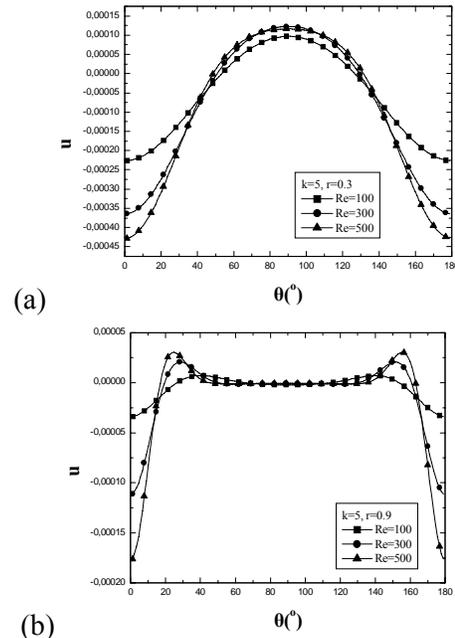
Fig. 8. (a) Variation of radial component of velocity with meridional coordinate near the inner boundary ( $r = 0.3$ ) for  $Re = 100, 300, 500$  and  $k = 5$ ; (b) Variation of radial component of velocity with meridional coordinate near the outer boundary ( $r = 0.9$ ) for  $Re = 100, 300, 500$  and  $k = 5$ .
