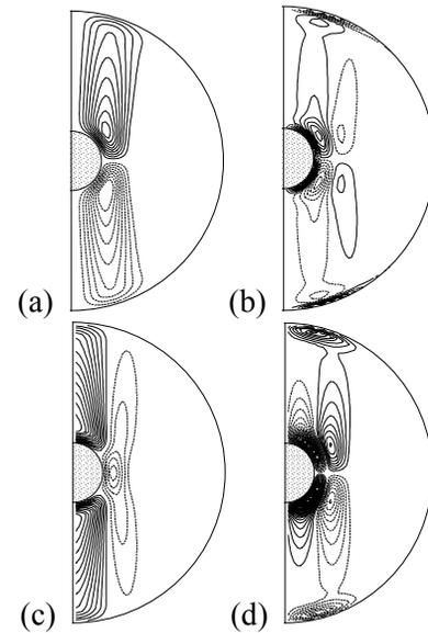
Fig. 5. Streamlines of the motion, function  $J$  of the vorticity, radial component of velocity and meridional component of velocity for  $Re = 800$  and  $k = 5$ .
