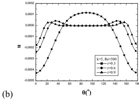
Fig.6. (a) Variation of radial component of velocity with radial distance at  $\theta = 2.25^\circ, 44^\circ, 88.88^\circ$  for  $Re = 500$  and  $k = 5$ ; (b) Variation of radial component of velocity with meridional coordinate  $\theta$  at  $r = 0.3, 0.6, 0.9$  for  $Re = 500$  and  $k = 5$ .
