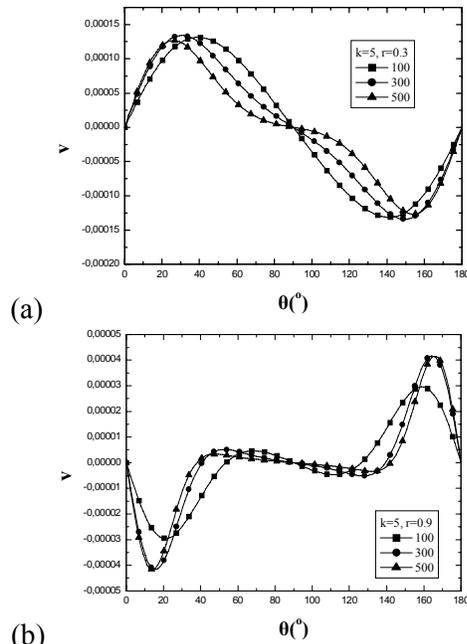
Fig. 9. (a) Variation of meridional component of velocity with meridional coordinate near the inner boundary ( $r = 0.3$ ) for  $Re = 100, 300, 500$  and  $k = 5$ ; (b) Variation of meridional component of velocity with meridional coordinate near the outer boundary ( $r = 0.9$ ) for  $Re = 100, 300, 500$  and  $k = 5$ .
