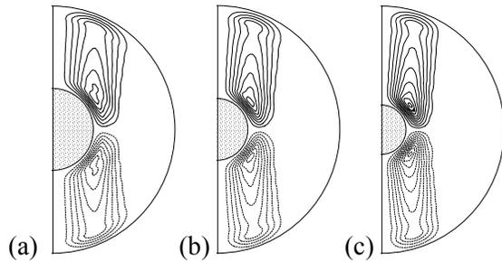
Fig. 3. Streamlines of the motion for  $Re = 500$  and (a)  $k = 3$ ; (b)  $k = 4$ ; (c)  $k = 5$ .
