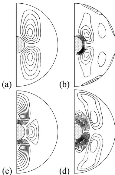
Fig. 4. Streamlines of the motion, function  $J$  of the vorticity, radial velocity and meridional velocity for  $Re = 100$  and  $k = 5$ .
