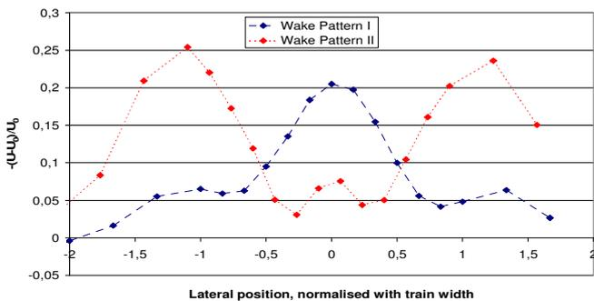
Fig. 3: Velocity profile in the wake of a train
