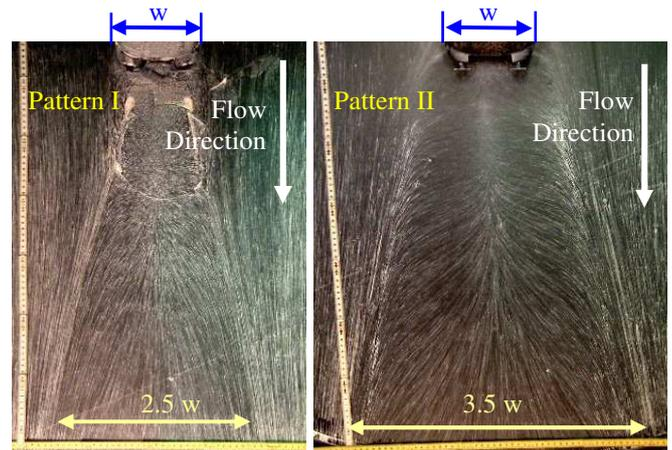
Fig. 5: Oil paint visualisation: footprints of the wake flow
