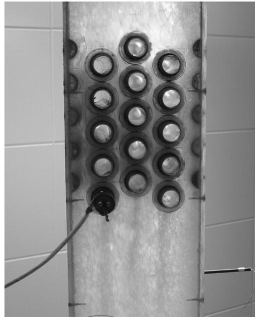
Fig. 3. Statically stable foam flow and tube bundle in the experimental channel
