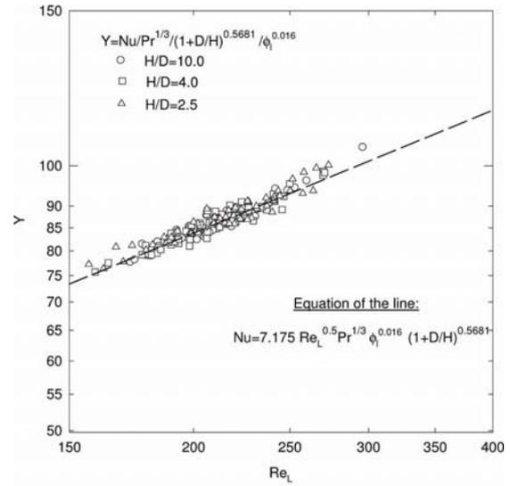
Fig.8 Generalized Plot:  $Y$  (as defined in plot) versus  $Re_L$
