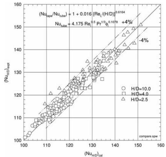
Fig. 9 Comparison between Calculated and Experimental Nusselt numbers for Twisted tape inserts
