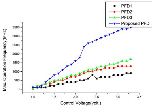
Fig. 7 Maximum operation frequency I
