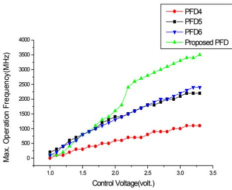
Fig. 8 Maximum operation frequency II
