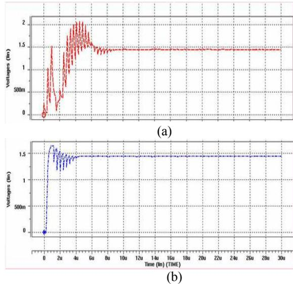
Fig. 15 Lock time comparison (a) without enhanced lock-in (b) with enhanced lock-in
