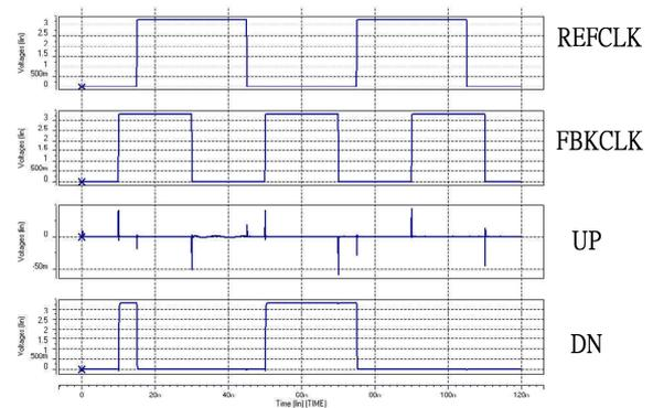
Fig. 6 Different frequency (REFCLK lags)
