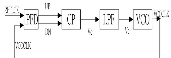
Fig. 1 Digital phase-locked loop
