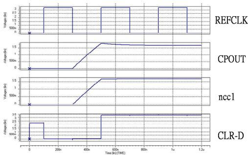
Fig. 13 Outputs of initial bias circuit for a reference input clock at 2.5MHz
