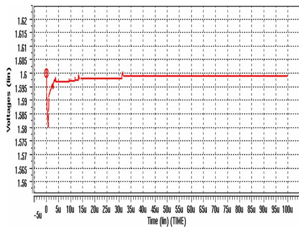
Fig. 11 1.1 GHz PLL whole loop function (Vc)
