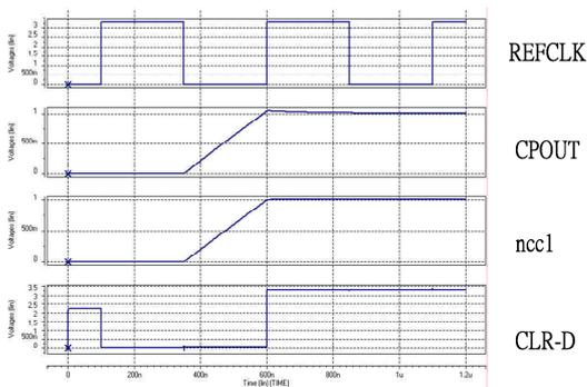
Fig. 14 Outputs of initial bias circuit for a reference input clock at 2.0MHz
