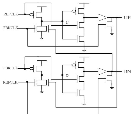
Fig. 3 Proposed high speed PFD
