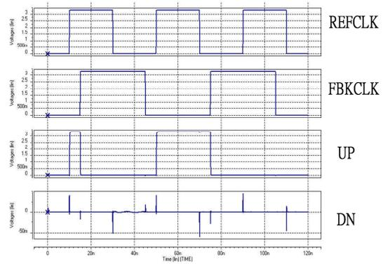
Fig. 5 Different frequency (REFCLK leads)
