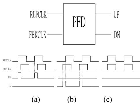
Fig. 2 Operation of PFD (a) lead (b) lag (c) in phase
