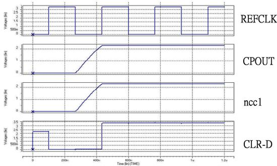
Fig. 12 Outputs of initial bias circuit for reference input clock at 3.0MHz
