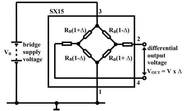
Fig. 1 The pressure transducer bridge arrangement
