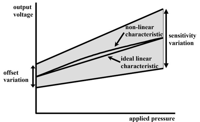
Fig. 2 Typical pressure transducer characteristics
