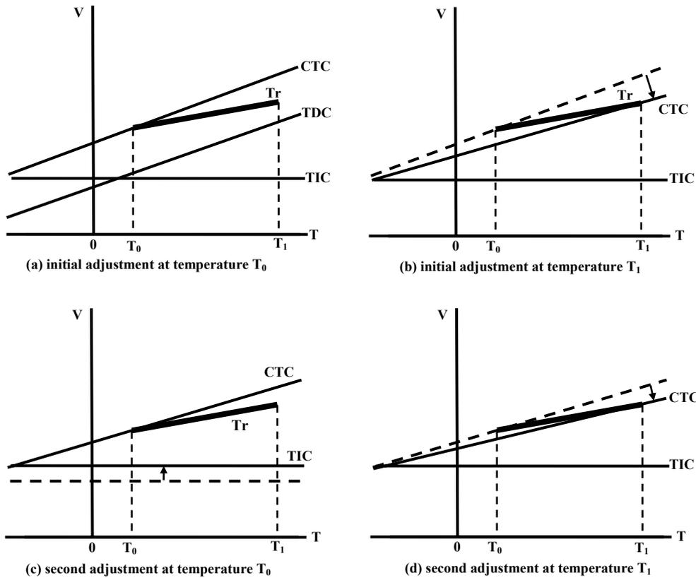
**Fig. 3** Adjustment of the temperature compensation mechanism for the transducer offset voltage
