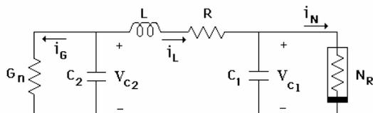
Fig.1. Chua's canonical circuit
