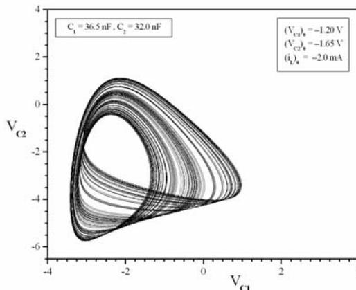
Fig.13. Chaotic spiral attractor for  $C_1 = 36.5$  nF,  $C_2 = 32.0$  nF and initial conditions  $(v_{C1})_0 = -1.20$ V,  $(v_{C2})_0 = -1.65$ V, and  $(i_L)_0 = -2.0$ mA
