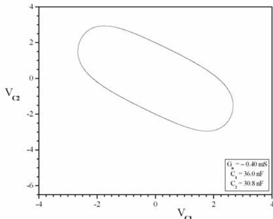
Fig.12. Phase portrait for  $C_1 = 36.0$  nF and  $C_2 = 30.8$  nF. Limit cycle.
