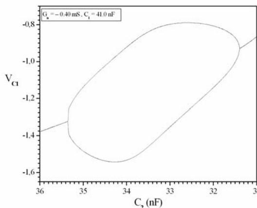
Fig.3. The bifurcation diagram,  $v_{C1}$  vs.  $C_2$ , for  $C_1 = 41.0$  nF.
