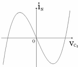
Fig.2. The cubic v-i characteristic of the nonlinear resistor.
