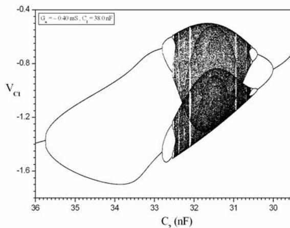
Fig.7. The bifurcation diagram  $v_{C1}$  vs.  $C_2$ , for  $C_1 = 38.0$  nF.
