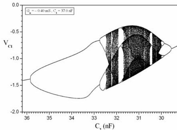
Fig.8. The bifurcation diagram  $v_{C1}$  vs.  $C_2$ , for  $C_1 = 37.0$  nF.
