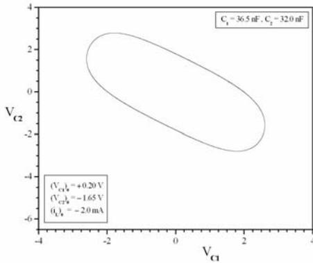
Fig.14. Period-1 limit cycle for  $C_1 = 36.5$  nF,  $C_2 = 32.0$  nF and initial conditions  $(v_{C1})_0 = +0.20V$ ,  $(v_{C2})_0 = -1.65V$ , and  $(i_L)_0 = -2.0mA$ .
