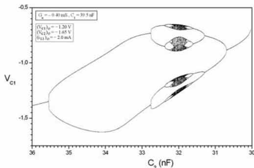
Fig.5. The bifurcation diagram  $v_{C1}$  vs.  $C_2$ , for  $C_1 = 39.5$  nF.
