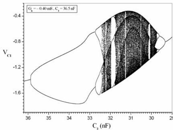
Fig.9. The bifurcation diagram  $v_{C1}$  vs.  $C_2$ , for  $C_1 = 36.5$  nF.
