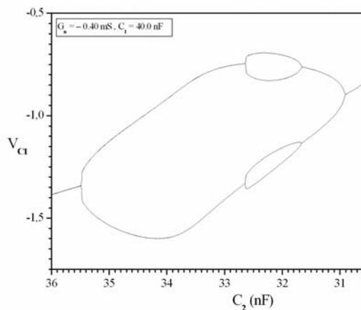
Fig.4. The bifurcation diagram,  $v_{C1}$  vs.  $C_2$ , for  $C_1 = 40.0$  nF.
