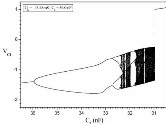
Fig.10. The bifurcation diagram  $v_{C1}$  vs.  $C_2$ , for  $C_1 = 36.0$  nF.
