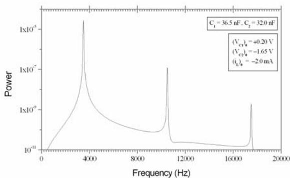
Fig.16. Power spectrum of the periodic attractor of Fig.14.
