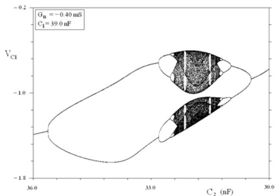
Fig.6. The bifurcation diagram  $v_{C1}$  vs.  $C_2$ , for  $C_1 = 39.0$  nF.
